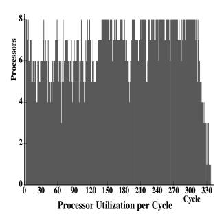
Figure 5: The result of scheduling the 9-body program onto eight Supercomputer Toolkit processors. Comparison with with the region-level parallelism profile (figure 4) illustrates how the scheduler spread the coarse-grain parallelism across the processors. A total of 340 cycles are required to complete the computation. On average, 6.5 of the 8 processors are utilized during each cycle.
