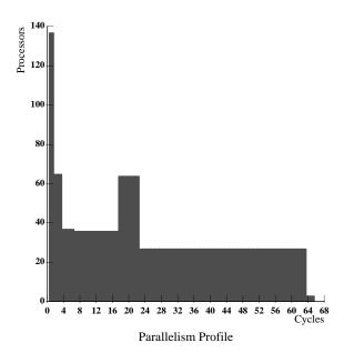
Figure 4: Parallelism profile of the 9-body problem after operations have been grouped together to form regions. Comparison with Figure 2 clearly shows that increasing the grain-size significantly reduced the opportunities for parallel execution. In particular, the maximum speedup factor dropped from 69 times faster to only 34.5 times faster than a single processor.
