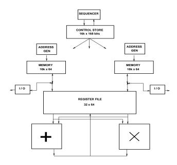
Figure 1: This is the overall architecture of a Supercomputer Toolkit processor node, consisting of a fast floating-point chip set, a 5-port register file, two memories, two integer alu address generators, and a sequencer.
