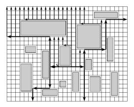
Figure 11: Operation of the ray algorithm.
