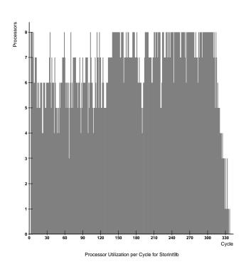
Figure 8: The result of scheduling the 9-body problem onto 8 Supercomputer Toolkit processors. Comparison with with the region-level parallelism profile (figure 6) illustrates how the scheduler spread the course-grain parallelism across the processors. A total of 340 cycles are required to complete the computation. On average, 6.5 of the 8 processors are utilized during each cycle.
