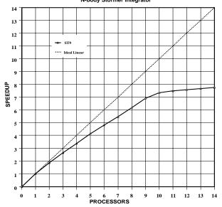
Figure 9: Speedup graph of Stormer integrations. Ample speedups are available to keep the 8-processor *Supercomputer Toolkit* busy, However, the incremental improvement of using more than 10 processors is relatively small.
