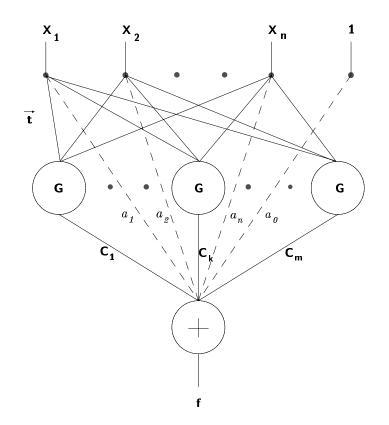
Figure 4: A network of the Hyper Basis Functions type. For object recognition the inputs could be image measurements such as values of different filters at each of a number of locations in the image. The network is a natural extension of the template matching scheme and contains it as a special case. The dotted lines correspond to linear and constant terms in the expansion. The output unit may contain a sigmoidal transformation of the sum of its inputs (see Poggio and Girosi, 1990b).
