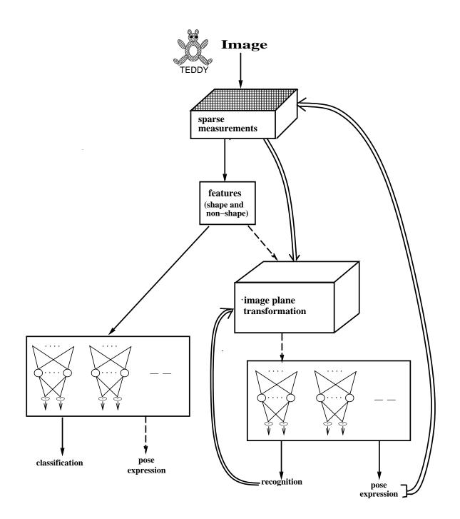
Figure 3: A sketch of possibly the most compact (but not the only!) implementation of the proposed recognition architecture in terms of modules of the HBF type.
