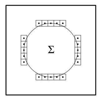
Figure 5: Motion detector that exploits Stokes' theorem.
