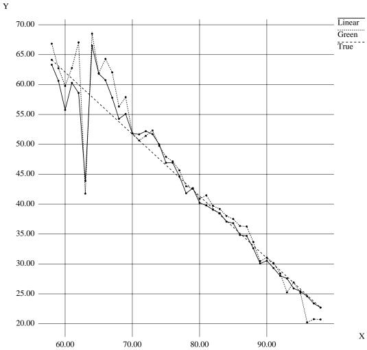
Figure 11: TTC measurements comparison by using 2D-2D and 1D-2D. In this and the following figures the abscissa gives the time in terms of elapsed frames; the ordinate gives the estimate of the time to crash in frame units.
