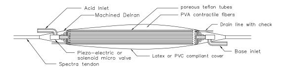
Figure 2-1. Two fluid microvalues meter desired amounts of acid or base through an irrigation system to a bundle of contractile fibers.
