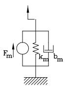
Figure 3-4. Simple model of contractile fiber.
