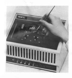
Figure 6-3: Alternate Cleaning of the EOT/BOT Sensor
