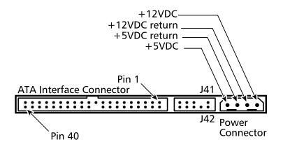
Figure 2-1 PCBA Jumper Location and Configuration
