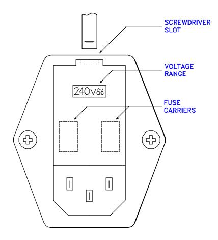
FIGURE B.1.2 VOLTAGE SETTING (I.T. MAINS)
