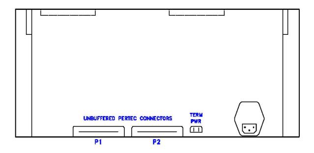
FIGURE 2.6.2 (a) CONNECTOR LOCATIONS, UNBUFFERED PERTEC
