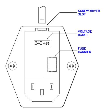
FIGURE 2.2.2 SUPPLY VOLTAGE SETTING
