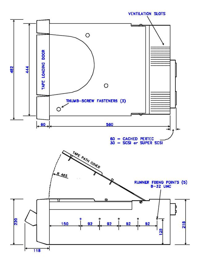
FIGURE 2.3(b) 9914 RUNNER FIXING POINTS
