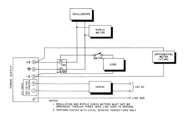
Figure 9. Test Connections for Performance Checks
