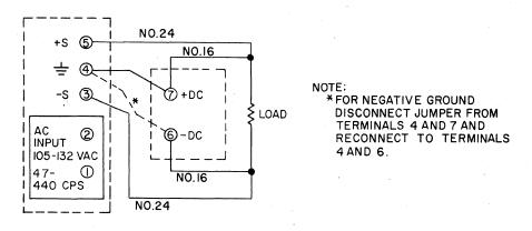
Figure 4. Remote Sensing Connections
