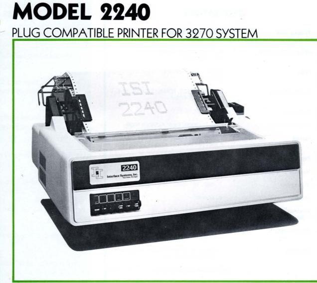
The model 2240 is plug compatible with your IBM 3270 communications system. It will replace the 328x without software changes. Just plug it in and run your application.
