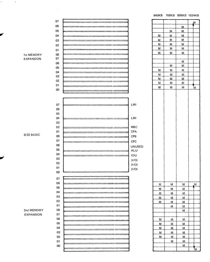
Figure 21. Front View of Processor Configuration with First and Second Memory Expansion
