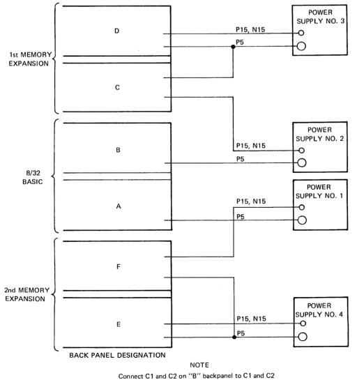
on "D" and "E" backpanels with jumper wires 17-372.
