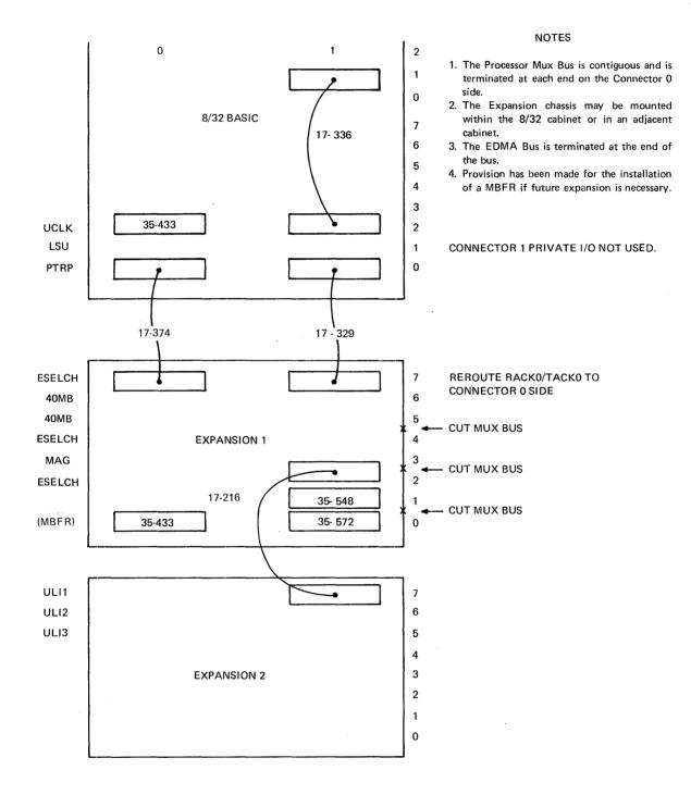
Figure 25. Typical System Configuration (Back Panel)
