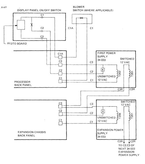
Figure 10. Set Up for Additional Power Supplies (34-033)
