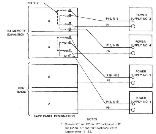
2. Remove P15 and N15 jumpers on backpanel "C" and "D".
