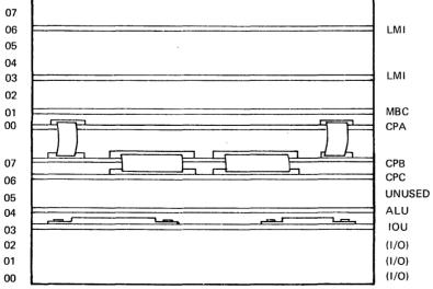
Figure 20. Front View of Processor Configuration with First Memory Expansion
