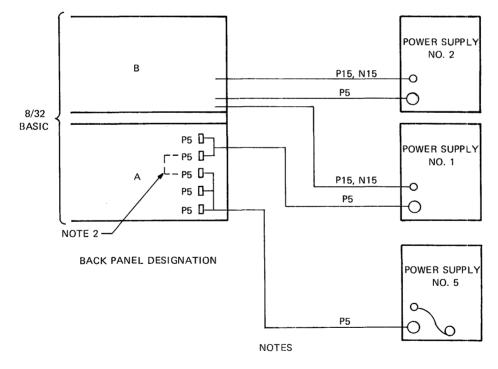
1. P15 and N15 voltages on this Power Supply must be adjusted to within a range of 15 to 17.5 volts to prevent crowbars from triggering.
