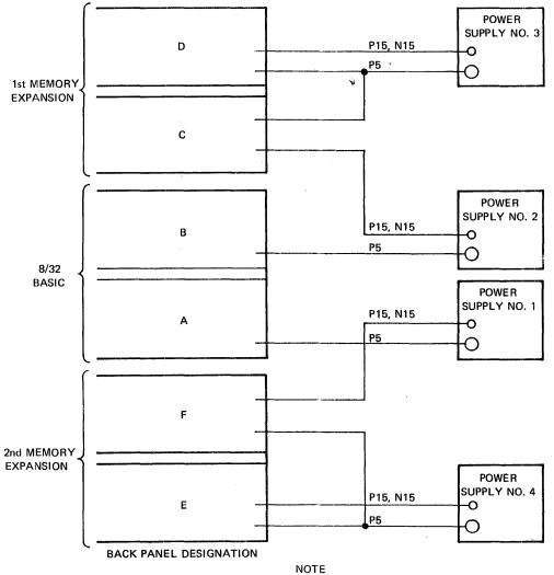
Connect C1 and C2 on "B" backpanel to C1 and C2 on "D" and "E" backpanels with jumper wires 17-372.
