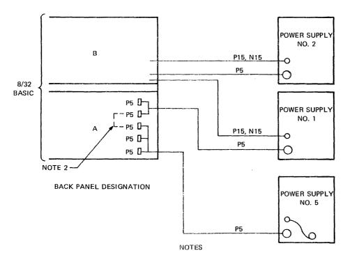
P15 and N15 voltages on this Power Supply must be adjusted to within a range of 15 to 17.5 volts to prevent crowbars from triggering.
