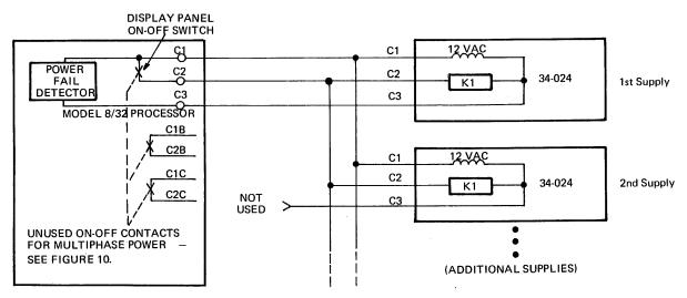
Figure 9. Power Control Circuit Diagram
