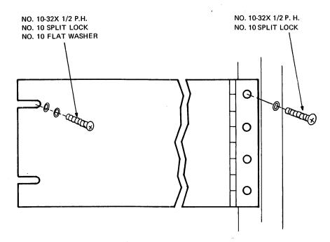
Figure 8. 34-024 Power Supply Mounting
