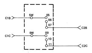
Figure 10. Wiring of the Second Deck of the Rotary Switch for Control of Different AC Phases
