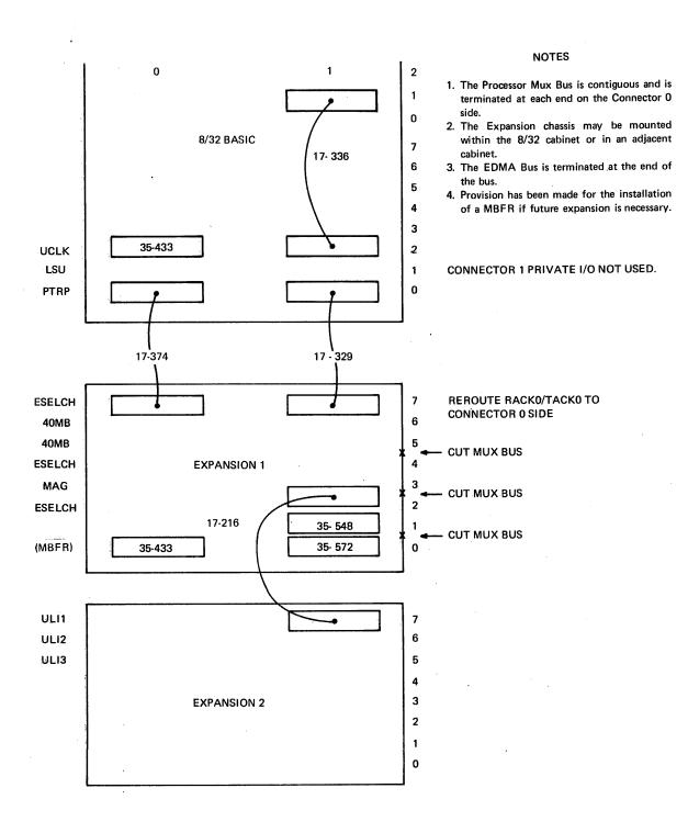
Figure 25. Typical System Configuration (Back Panel)
