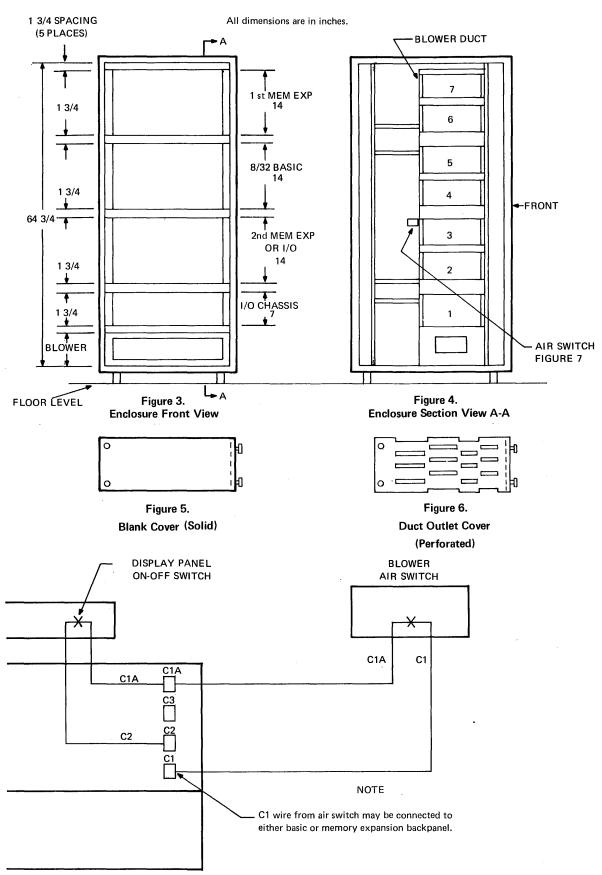
Figure 7. Wiring of the Blower Air Switch
