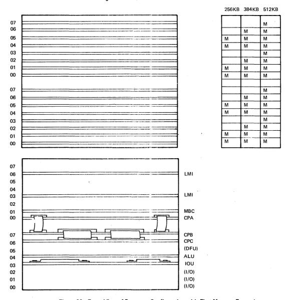
Figure 20. Front View of Processor Configuration with First Memory Expansion
