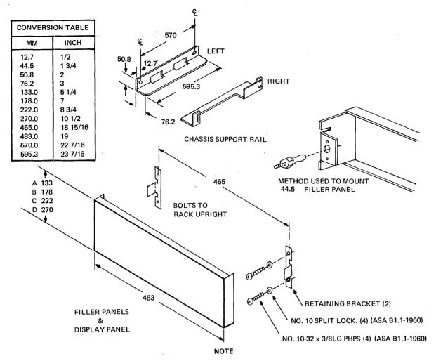
All dimensions are in millimeters unless otherwise specified. Use table for conversion to English units.
