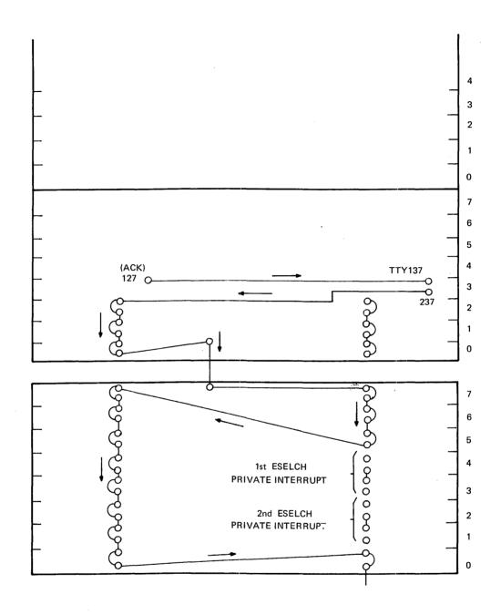
Figure 24. Interrupt Priority with ESELCH Installed
