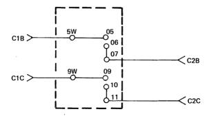
Figure 10. Wiring of the Second Deck of the Rotary Switch for Control of Different AC Phases
