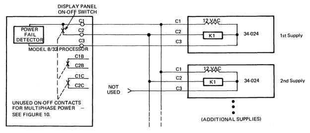
Figure 9. Power Control Circuit Diagram
