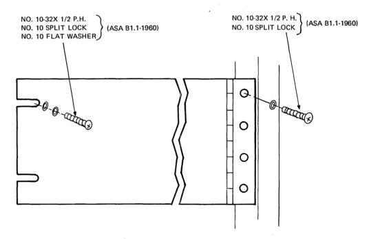
Figure 8. 34-024 Power Supply Mounting
