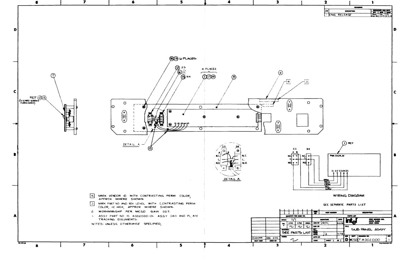
Figure 4-3. iSBC 655 Sub Panel Assembly
