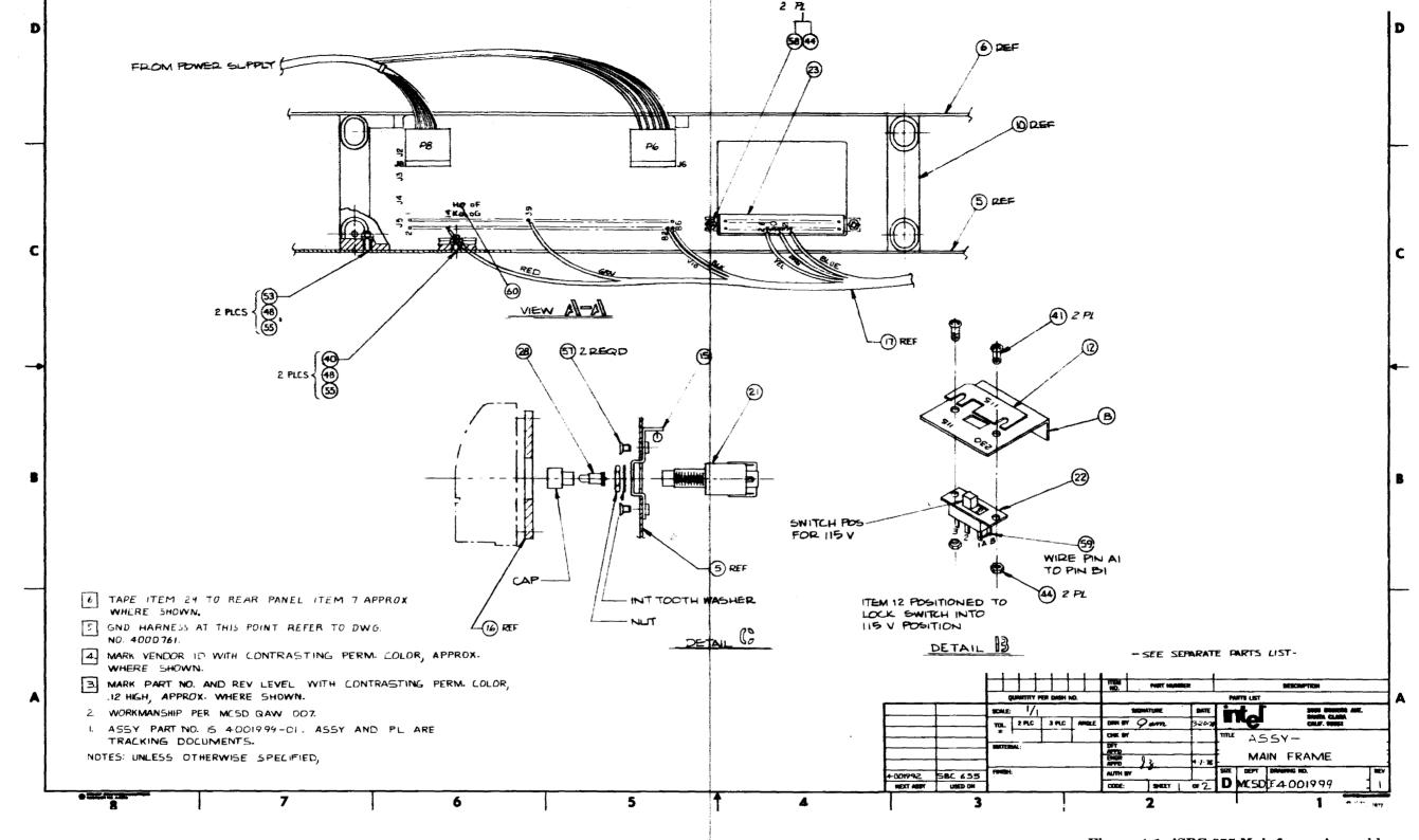
Figure 4-1. iSBC 655 Mainframe Assembly (Sheet 1 of 2)
