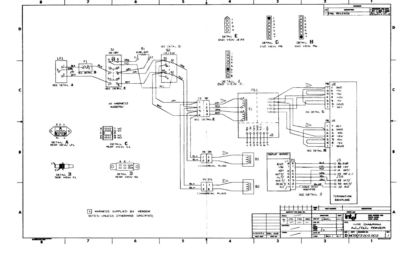
Figure 4-2. iSBC 655 Wiring Diagram
