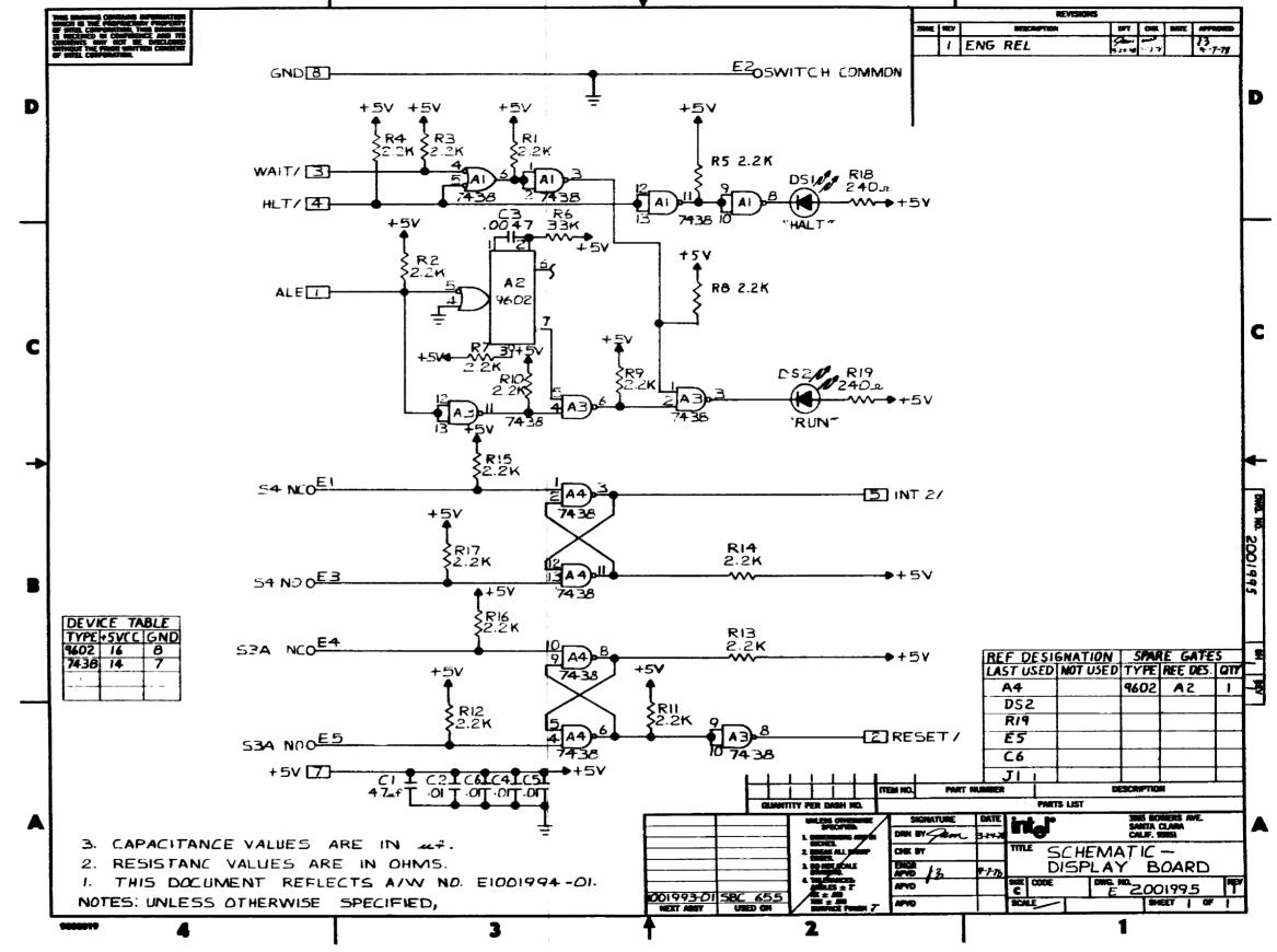
Figure 4-5. iSBC 655 Display Board Schematic
