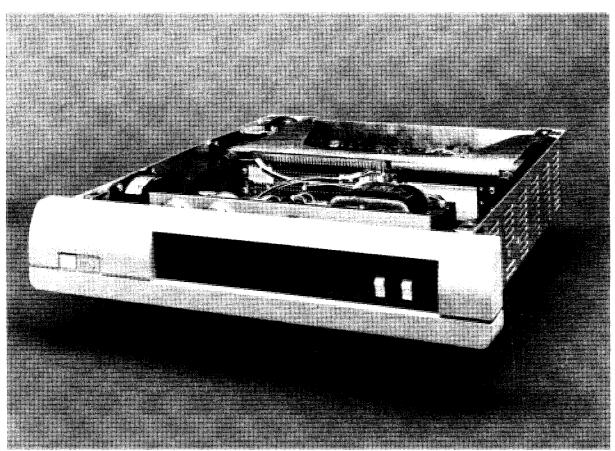
Figure 1-1. iSBC 655 System Chassis
