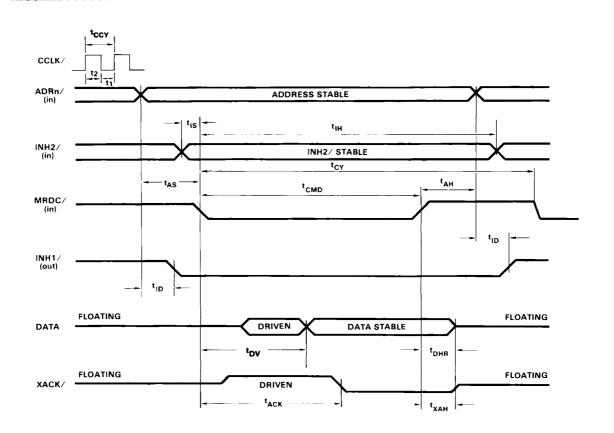
Figure 2-1. Bus Exchange Timing
