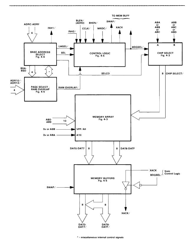
Figure 3-1. iSBC\*\* 464 Board Functional Block Diagram
