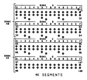
Figure 2-2. Base Address Select Jumpers
