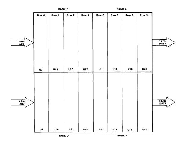
Figure 3-2. Memory Array Functional Layout
