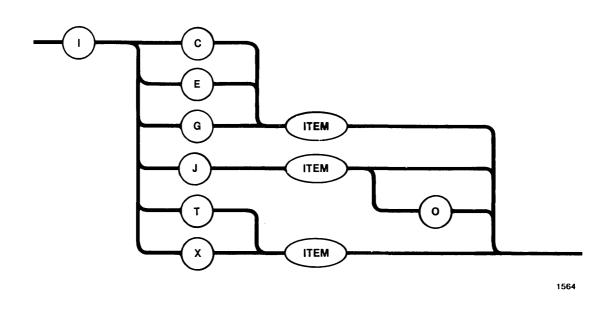
Figure 4-2. Syntax Diagram for Inspecting System Objects
