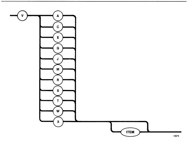
Figure 4-11. Syntax Diagram for Viewing iRMX<sup>®</sup> I Object Lists
