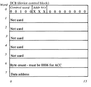
Figure 2-3. Format of the DCB for a start cycle steal status command
