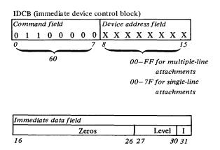
Level. This four-bit encoded field specifies the priority interrupt level assigned to the device.
