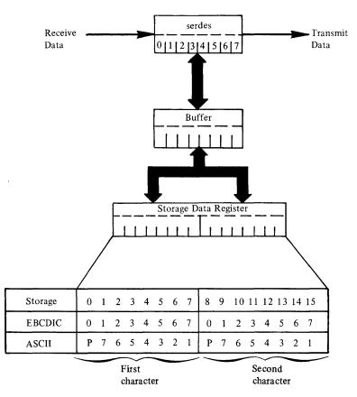
Figure 4-1. SDLC Attachment Data Flow
