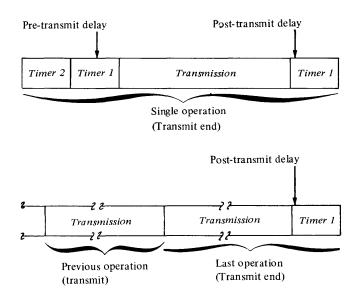
**Transmit Allow Break.** This operation is the same as the *Transmit* operation, except that it allows the receiving station to stop the transmission. To do this, the receiving station "breaks" the line for at least 150 milliseconds. If the attachment detects this condition, it resets transmit mode and 'request to send', and presents an exception interrupt with bit 0 on in the Interrupt Status Byte. The attachment does not reset RTS if it is permanently jumpered "on."
