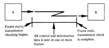
The higher level of grouping, a frame sequence, is checked by the software for missing or duplicated frames. The software at a station transmitting sequenced frames counts and numbers each sequenced frame. This count is known as Ns. The software at a station receiving sequenced frames counts each error-free sequenced frame that it receives; the receiver count is called Nr.
