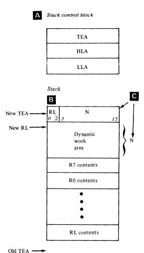
Figure 2-5. Word stack for subroutine linkage
