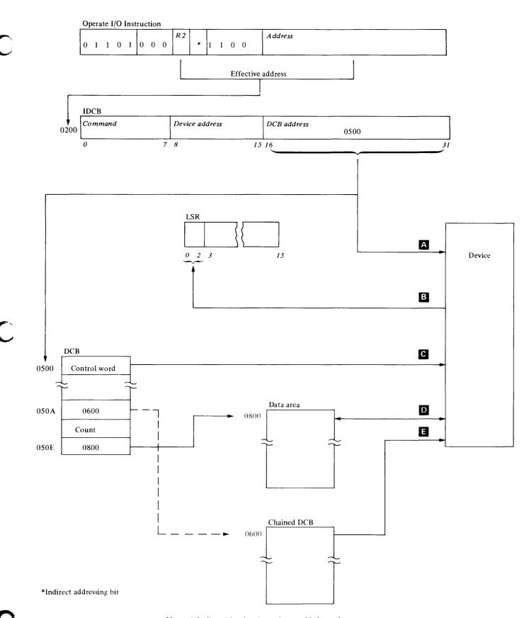
Figure 4-5. Example of cycle steal control information
