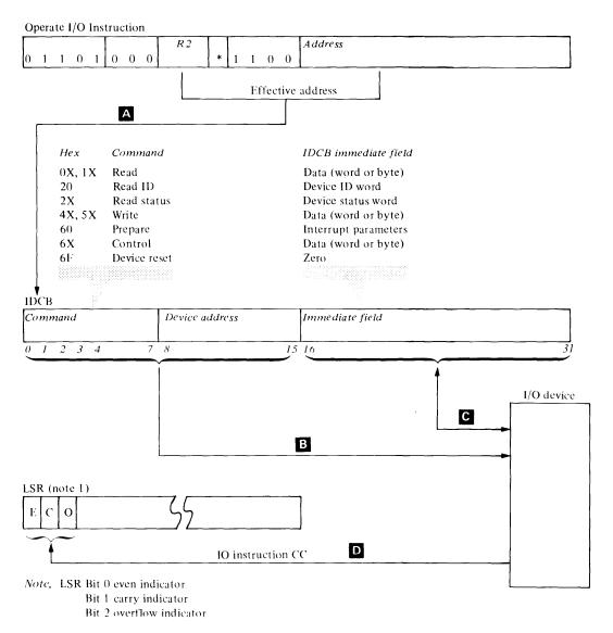
Figure 4-4. Direct program control I/O operation
