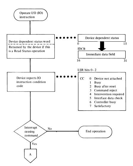
Figure 4-7. Condition codes, status words, and status bytes received from a device (Part 1)
