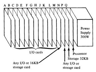
If the A position is not used for the Channel Repower card, the following feature cards may be plugged in this position:
