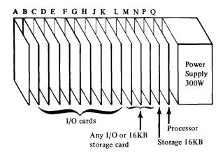
If the A position is not used for the Channel Repower card, the following feature cards may be plugged in this position:
