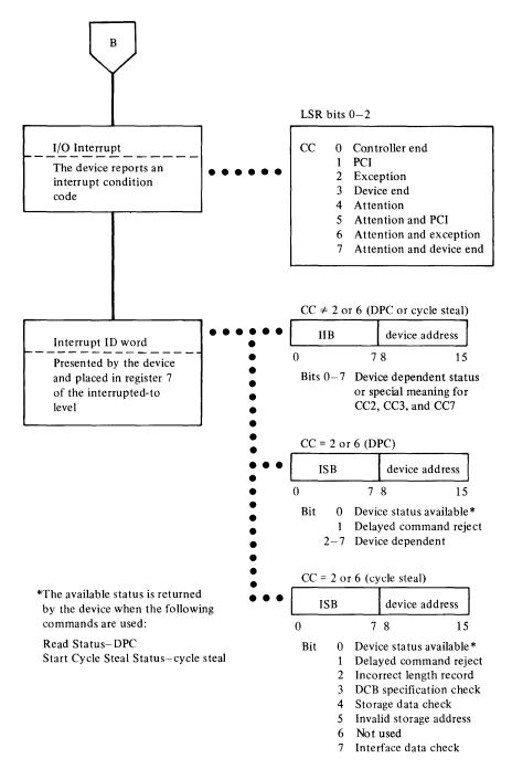
Figure 4-7. Condition codes, status words, and status bytes received from a device (Part 3)
