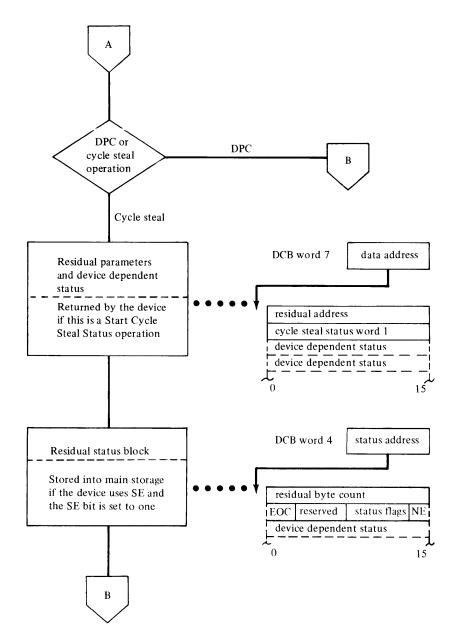
Figure 4-7. Condition codes, status words, and status bytes received from a device (Part 2)
