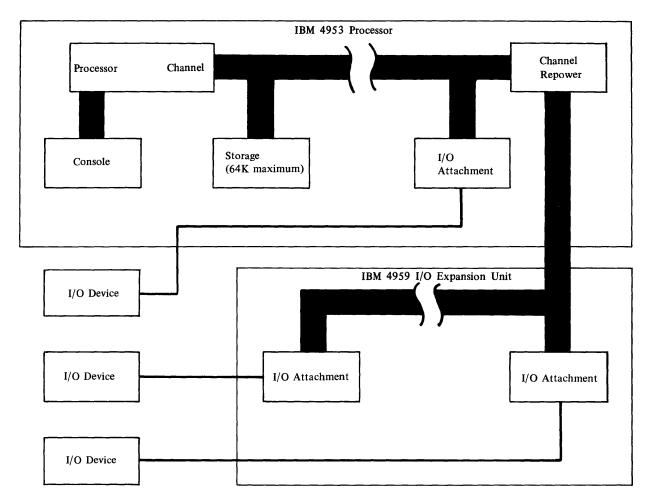
Figure 1-1. Block diagram of IBM 4953 Processor and an IBM 4959 I/O Expansion Unit
