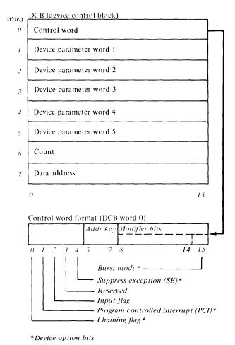
Figure 4-3. Device control block
