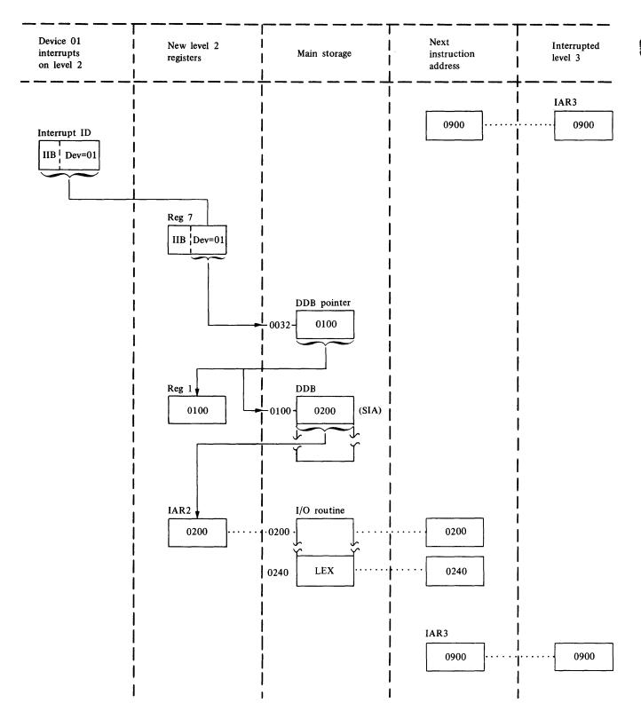
Figure 3-3. Example of I/O interrupt with automatic branching
