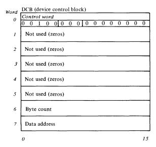
Figure 4-6. DCB for start cycle steal status operation
