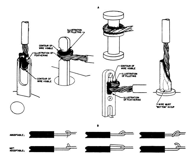
Figure 1-2. Correct and Incorrect Soldering Connections
