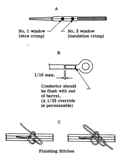
Figure 4-1. Cabling Crimps and Hitches
