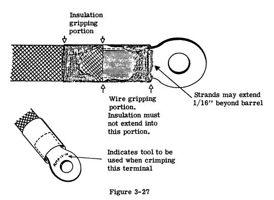
(8) The wire shall be inserted in the barrel of the connector so that the area of contact after crimping is equal to or greater than the cross section area of the wire.
