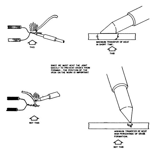
Figure 1-3. Correct and Incorrect Soldering Methods
