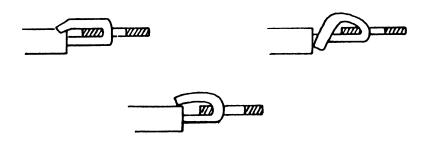
Unsatisfactory Mechanical Wraps on Eyelet Type Terminals
