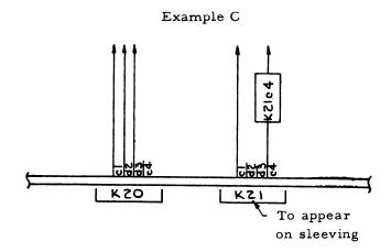
Figure 4-6. Wire Marker Identification
