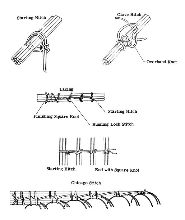
Figure 4-2. Lacing Stitches and Knots
