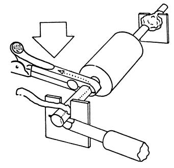
Electrical components that may be adversely affected by excessive heat should be protected by a heat shunt.
