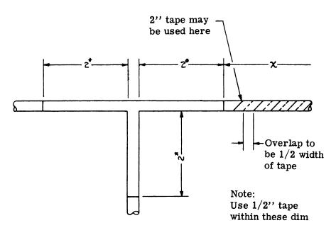
Figure 4-5. Taping
