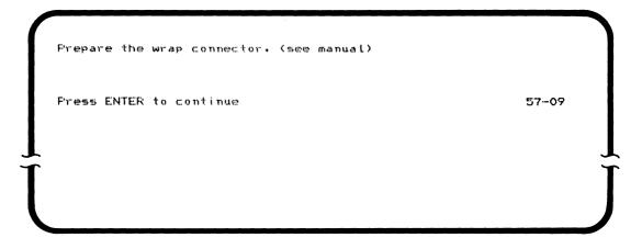
Obtain the 15-pin wrap connector from the Verification binder. The binder contains two connectors. Use the 15-pin connector for this portion of the test. Disconnect the cable from the channel service unit (CSU). Put the wrap connector on the end of the cable. Press the ENTER key.
