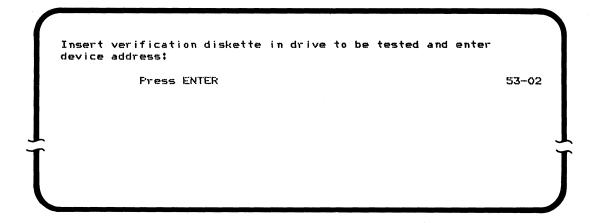
9. Move the verification diskette to the drive to be tested if necessary, and enter the device address of the diskette drive to be tested. Press the ENTER key.
