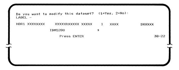
Note: If you press the HOME key when the first data set label is shown on screen, the volume label is displayed. you press the HOME key when any other data set label is shown, the preceding data set label is displayed.
