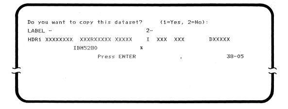
Note: If you press the HOME key when the first data set is shown on the screen, the volume label is displayed. If you press the HOME key when any other data set label is shown, the preceding data set label is displayed.
