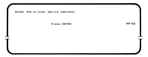
4. Enter the device address of the printer, and press the ENTER key.
