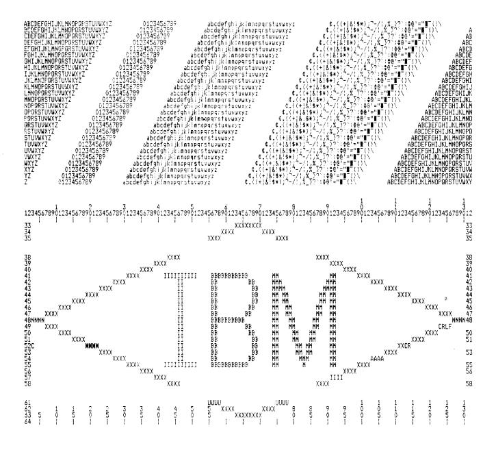
Note: This test pattern is printed to ensure that the printer interface is operating correctly. The style of the characters, and the characters that are printable, vary depending on which printer is being tested. Because of this, the characters in the test pattern printed on your printer might not match exactly the characters shown in this figure. However, the pattern itself should be correct.
