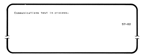
This display may stay on the screen for as long as 30 seconds. If the display does not change after that time, an error has occurred from which the system cannot recover. Call your service representative.
