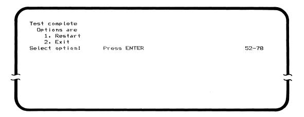
7. You may test other keyboards and any magnetic stripe readers by selecting option 2 which takes you back to the prompt for program name. At the next keyboard, repeat "Part 1 (Keyboard)" on page 14. Continue repeating this part until you have completed testing all keyboards.
