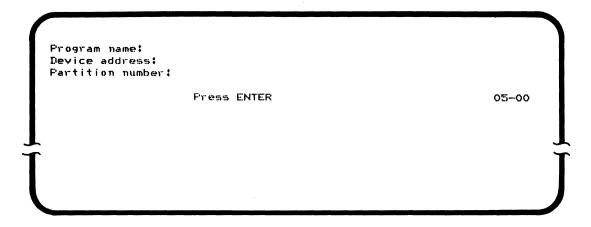
3. Enter the program name TKBD and press the FIELD+ or the FIELD EXIT key. If you cannot enter the program name, go to "BRANCH C" on page 17, step C2.
