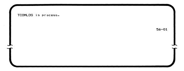
After the error log is written on the diskette, TSYSLOG is automatically loaded to save the system errors in the communications log area. See "How to Dump the System Error Log (TSYSLOG)" on page 57 for the prompts and instructions.
