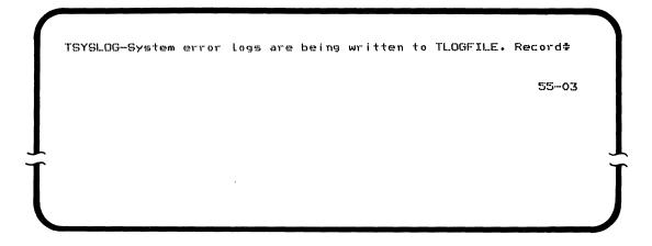
The record number on the display changes as the error logs are dumped to diskette.
