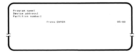
3. Enter the program name SYSDUMP, and press the FIELD+ or FIELD EXIT key.
