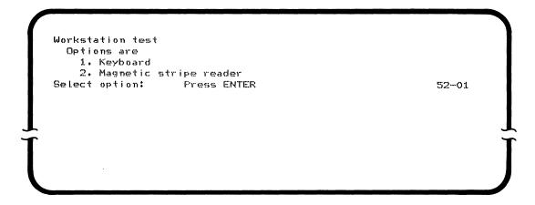
6. Select the option for the test you want, and press the ENTER key. If you choose option 1, Keyboard, continue in "Part 1 (Keyboard)" If you want to test only the magnetic stripe reader, option 2, go to "Part 2 (Magnetic Stripe Reader)" on page 16 of this procedure.
