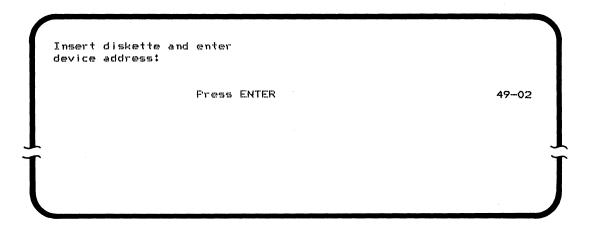
2. Insert a diskette that is initialized to a 128-byte record format, and does not contain data sets. Enter the address of the diskette drive being used.
