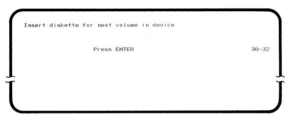
Note: Each additional output diskette or disk must have the same sector size and exchange type support as the first output diskette or disk.
