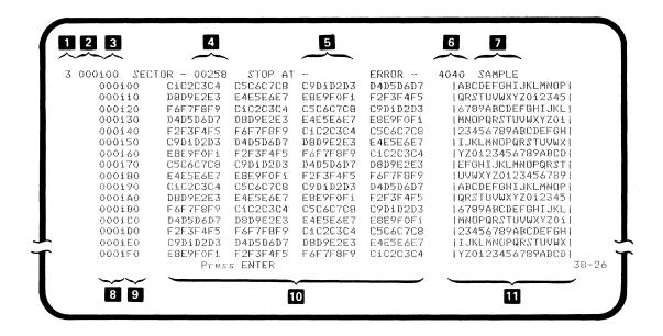
Note: The data in the data set record is displayed by disk sector. Each disk sector is 256 bytes long. A data set record may be less than, or greater than, 256 bytes and can overlap sector boundaries. If the system is unable to recover data from the disk, the data fields contain all dashes (hex 60).
