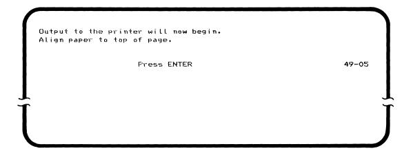
6. The memory dump is printed on the printer you specified. When it has completed, the following prompt is displayed:
