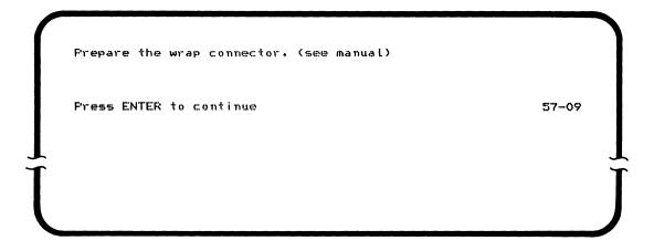
Obtain the wrap connector from the Verification binder. Disconnect the communications cable from the modem. Put the wrap connector on the end of the cable. Press the ENTER key. 15. If you encounter an error while running this test, remove the connector from the communications socket on the back of the controller and replace the cable with the wrap connector as shown.
