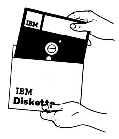
Return the diskette to its protective envelope whenever it is removed from the diskette drive and whenever you are writing on a label on the diskette.
