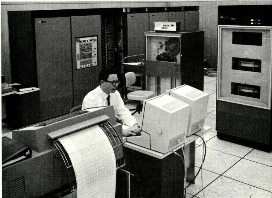
Figure 1-8. MTDS Data Acquisition and Control System with Peripheral Equipment
