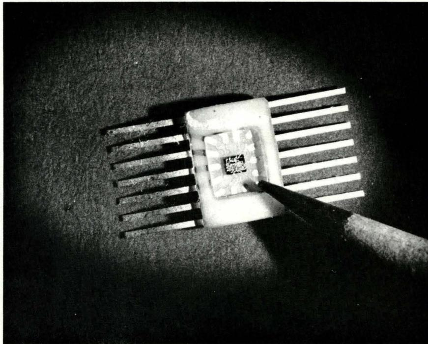
Figure 1-1. TTL Integrated Circuit
