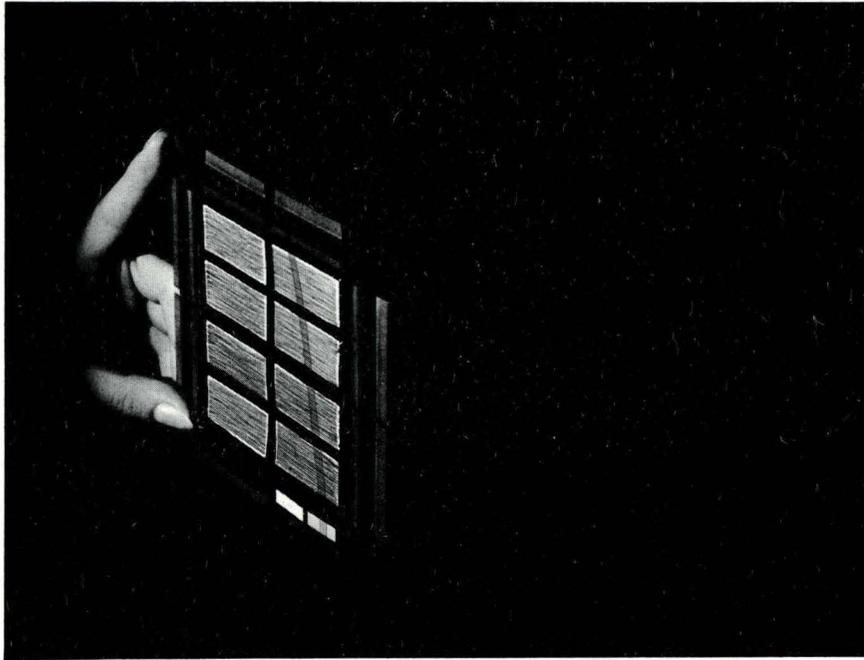
Figure 1-4. Main Storage Core Plane
