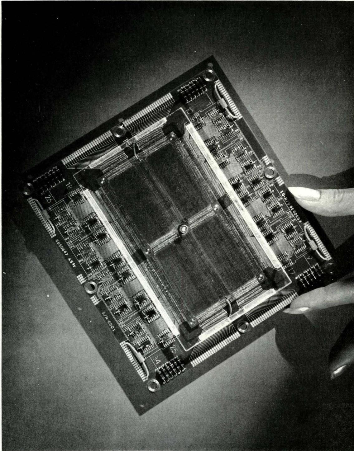
Figure 1-7. ROS Plane With Associated Electronics
