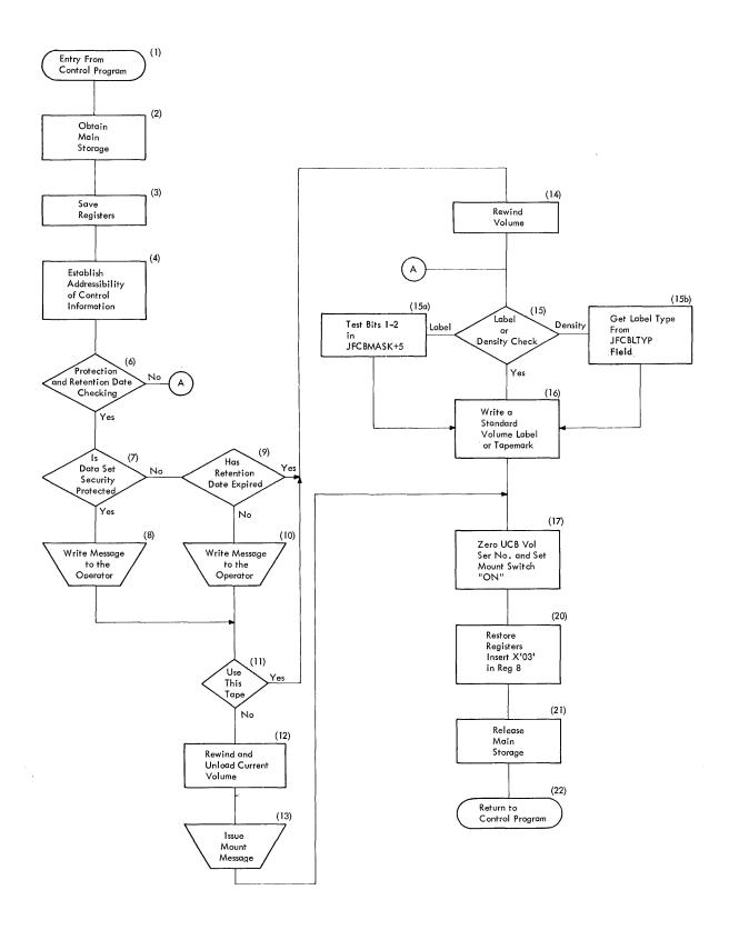
Figure 8. General Flow of an Editor Routine After Receiving Control From the End-of-Volume Routine
