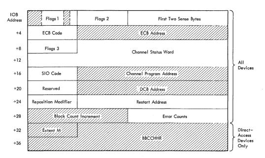
Figure 10. Input/Output Block Format
