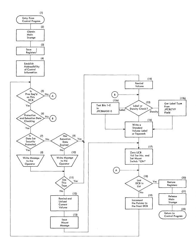
Figure 7. General Flow of an Editor Routine After Receiving Control From the OPEN Routine
