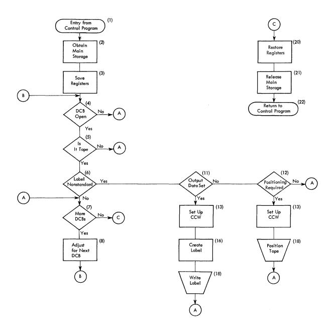
Figure 4. General Flow of a Nonstandard Label Processing Routine After Receiving Control From the CLOSE Routine
