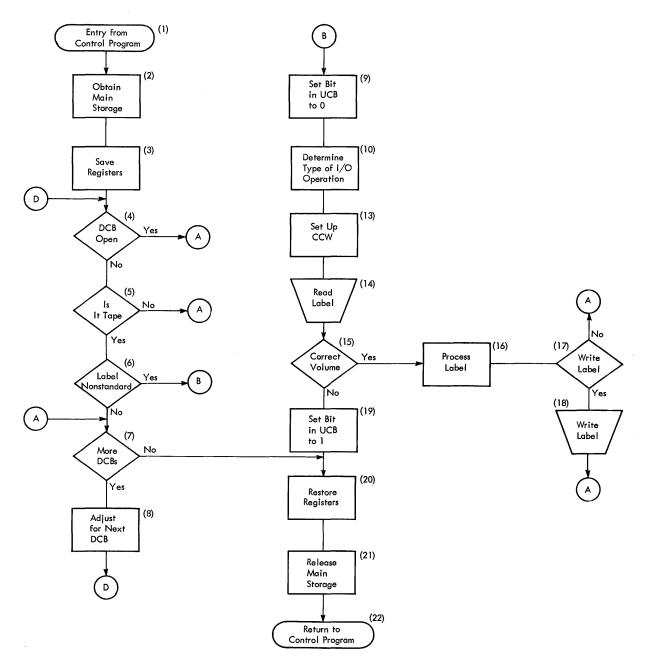
Figure 3. General Flow of a Nonstandard Label Processing Routine After Receiving Control From the OPEN Routine
