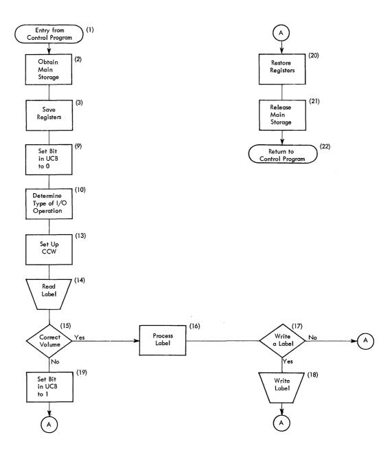
Figure 5. General Flow of a Nonstandard Label Processing Routine After Receiving Control From the EOV Routine
