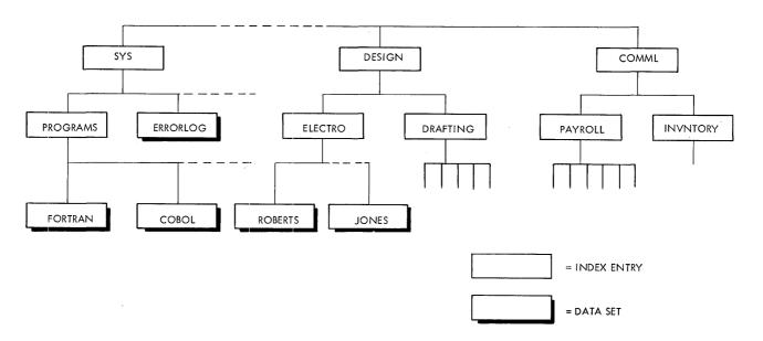
Figure 3. Simplified Diagram of a Catalog Organization
