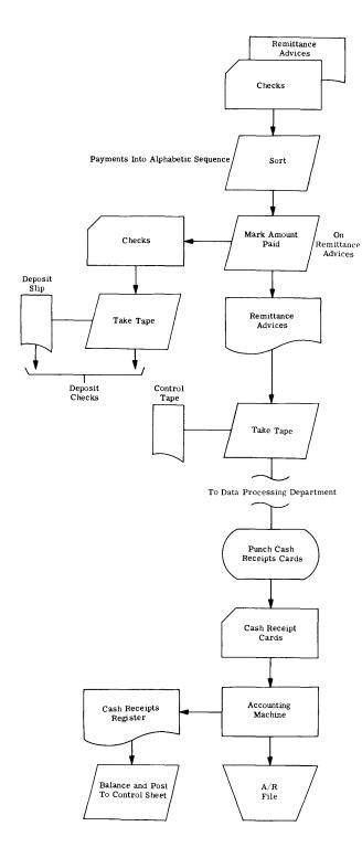
Figure 19. Punched card conventional approach -- balance-forward
