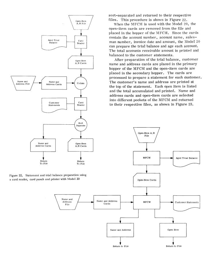
Figure 23. Statements and aged trial balance preparation using the Model 20 with the MFCM -- open-item
