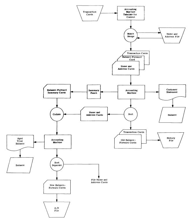
Figure 21. Punched card conventional approach -- balance-forward
