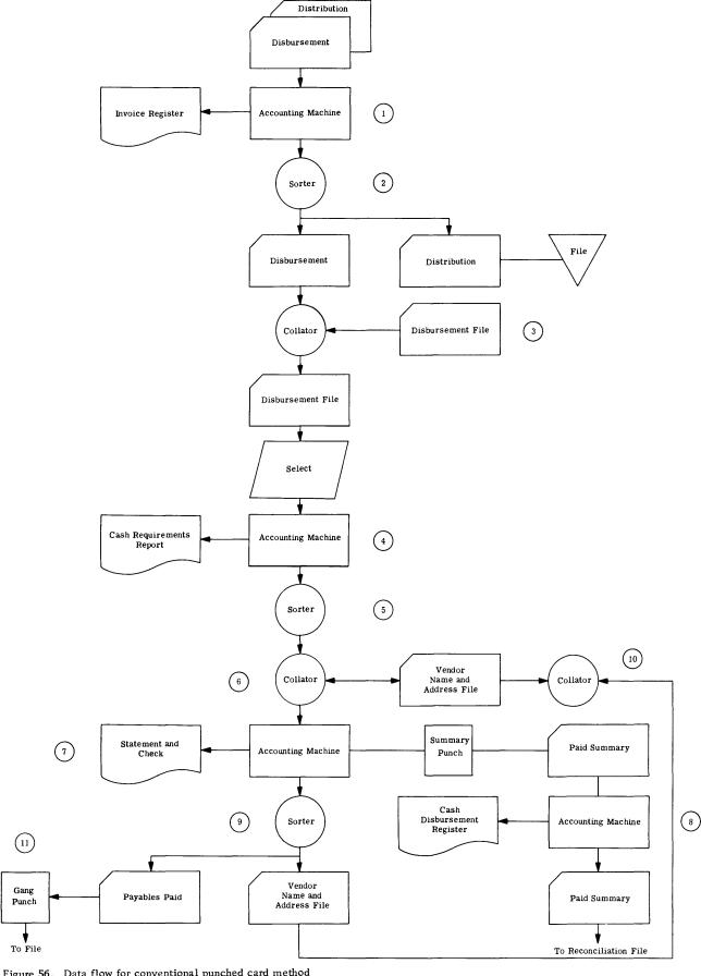
Figure 56. Data flow for conventional punched card method
