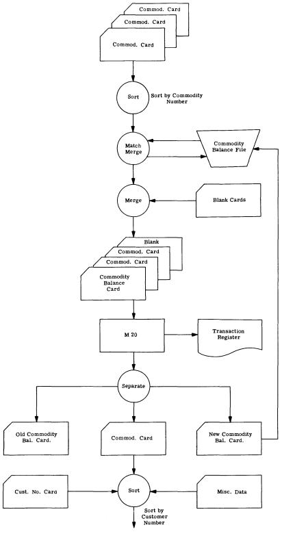
Figure 7. Batch billing with the card reader, punch and printer (1 of 2)
