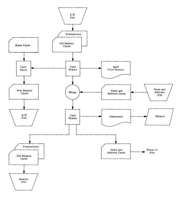
Figure 24. Statements and aged trial balance preparation using Model 20 with card reader, card punch and printer
