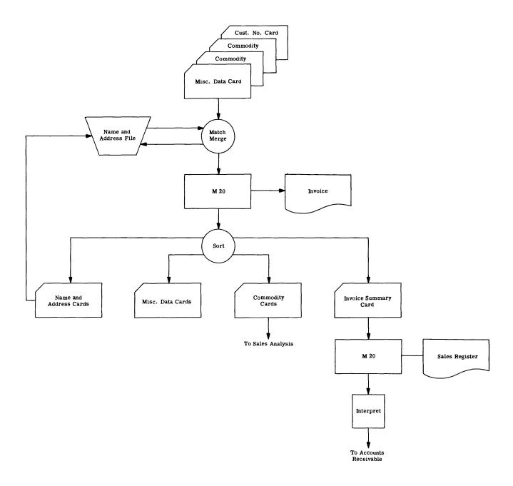
Figure 7. Batch billing with the card reader, punch and printer (2 of 2)
