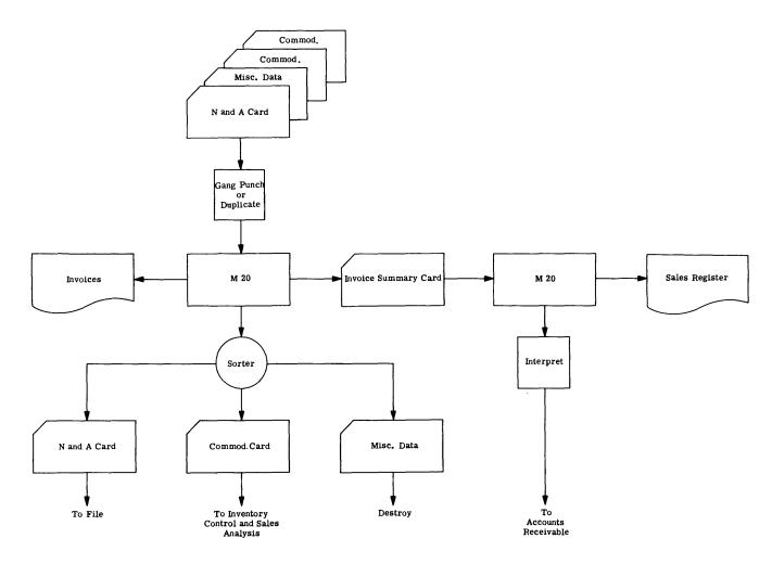
Figure 3. Billing with preassembled cards using the card reader, punch and printer
