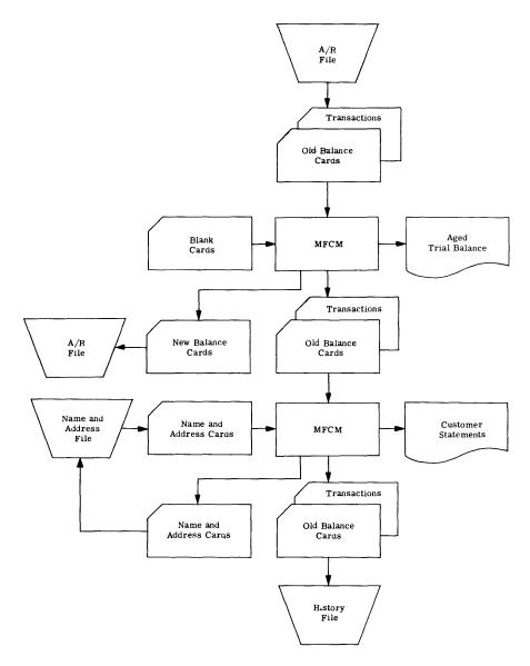
Figure 25. Statements and aged trial balance preparation using the Model 20 with the MFCM balance-forward
