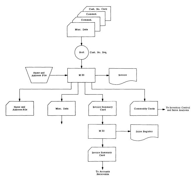
Figure 5. Billing using the MFCM and printer
