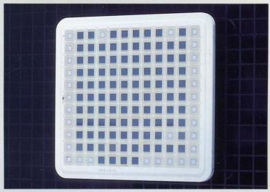
High density packaging techniques provide the potential for 132 logic and support chips to be packaged on this multi-layer ceramic substrate. This is the highest logic density package in the industry.
