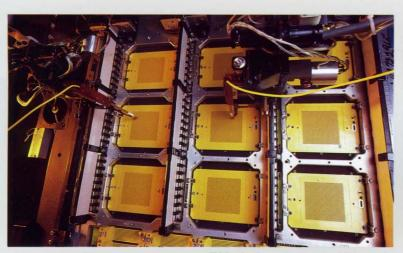
IBM robotic systems are widely used in production and testing of the 3090 TCM boards.
