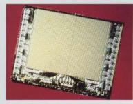
This IBM-developed and built, fast static random access memory (SRAM) chip is used in the 64Kbyte high-speed buffer which is attached to each central processor in an IBM 3090. The high-speed buffer, which is dynamically managed by hardware, and is transparent to programs, substantially improves system performance.
