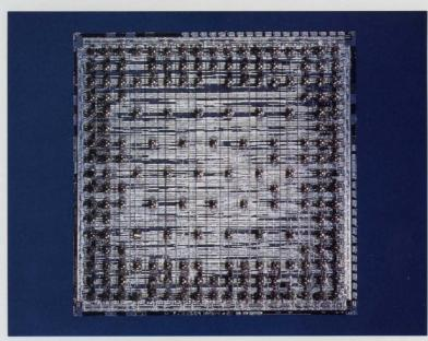
Fast bipolar emitter-coupled logic (ECL) chips allow the reduction in central processing cycle time on 3090 models compared to 308X models.
