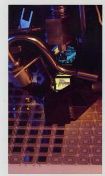
Logic and array chips are mounted on multilayer ceramic substrates and bonded using the IBM-invented C4 process.
