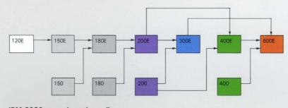
IBM 3090 upgrade options allow up to ten-fold growth in processor power.
