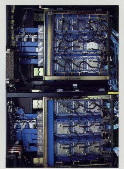
The central processor board in the triadic (300E) configuration is located above the Vector Facility board. Nine Thermal Conduction Modules (TCMs) make up each IBM 3090 Vector Facility board. Three TCMs are required for each Facility, and three Facilities are accommodated on each TCM board.
