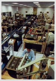
TCM boards are delivered and transferred automatically to work stations by the car-on-track conveyor system for greater operator safety and efficiency.
