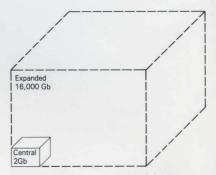
Expanded storage, using a 32-bit addressing structure, extends the system's processor storage capability to over 4 billion 4K pages, or 16 trillion bytes — many times the on-line data in a typical large system installation.
