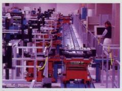
Parts move to people in the board assembly area on specially-built transport systems.
