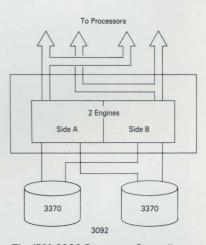
The IBM 3092 Processor Controller can contain one (on the 120E) or two independent processor engines. On the 3092 diagram shown above for a 3090 model 400E or 600E, one is in the active state, monitoring the IBM 3090 processor complex, the other is in standby ready to take over should the active one fail. Also, all key information recorded is duplicated on the two IBM 3370 disks which are connected to both processor engines in the 3092.
