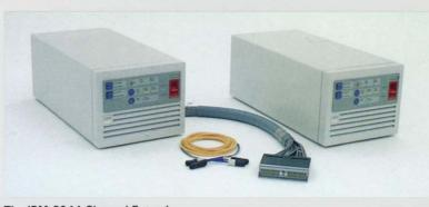
The IBM 3044 Channel Extender allows a channel to be extended up to 2km (6600 ft) at speeds up to 1.25 Mb/sec using fiber optic serial channels.
