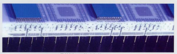
Multiple layers of buried wiring are revealed in this cutaway view of the substrate. The wires interconnect the chips soldered onto the surface using the special IBM-developed C4 process, resulting in high interconnection reliability and density.
