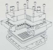
IBM-developed C4 interconnection technique, the 36-layer ceramic substrate, and the water-cooled TCM, IBM engineers have solved the difficult problem of packaging dense logic chips closer together for faster switching speeds, while at the same time providing a reliable method for efficient heat removal.
