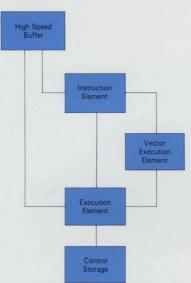
A Vector Facility is attached to the instruction and execution elements of a 3090 central processor. The instruction element fetches and decodes all the instructions including any vector instructions that are in the instruction stream. The instruction and execution elements access control storage, much as they do in System/370 operations, and then transfer the operands to or from the Vector Facility.
