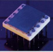
After the chips have been placed on the ceramic base, the chips "ride" the substrate through a furnace with tightly controlled temperatures. When the substrates emerge, the C4 "dome" has "reflowed," and each is now a highly reliable soldered connection.
