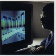
An IBM designer uses an IBM 5080 display to view a specially-developed three-dimensional model closeup of a cutaway Thermal Conduction Module (TCM). Extensive design using sophisticated imaging techniques results in highly reliable packaging for the IBM 3090.
