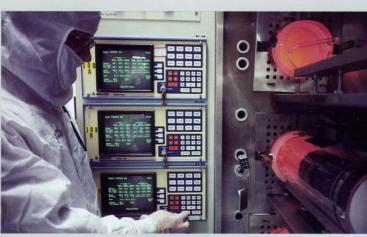
Round wafers of ultra-pure silicon are placed in an oxidation oven, which deposits a layer of silicon dioxide on which each layer of circuitry will be etched.
