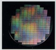
This wafer, 125 mm (five inches) in diameter contains approximately 150 of the newest IBM one-million-bit memory chips. To further enhance manufacturing productivity, IBM is first in the industry to phase in production of these advanced chips on 200 mm (eight-inch) wafers. The new 200 mm wafers can hold almost three times as many chips as the 125 mm wafer.
