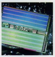
IBM-developed and built onemillion-bit memory chips are used in the 3090 processors. This first generation IBM 1-megabit chip is used in 3090 expanded storage.
