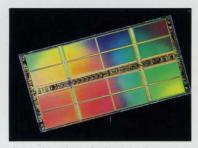
A combination of advances in manufacturing technology, circuit design, and chip architecture have made this chip — used for central storage in the IBM 3090 — one of the fastest, most advanced one-million-bit memory chips in the industry.
