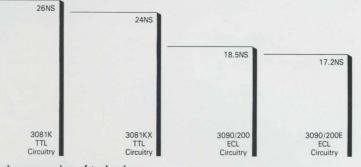
A steady progression of technology and design enhancements have allowed the machine cycle times on IBM large processors to continue to improve.
