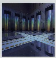
Extensive upgrade options are made possible in part by the extendibility of the 3090 advanced packaging technology as shown by this threedimensional computer-generated closeup of a cutaway Thermal Conduction Module.
