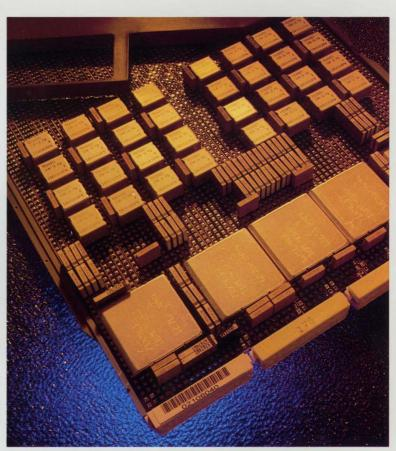
Four megabytes of memory can be stored in this field-replaceable circuit card.
