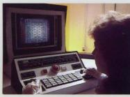
An IBM-designed closed circuit television system enables the operator to carefully align the chips before they are bonded to the ceramic substrate.
