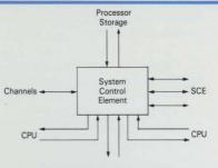
The System Control Element accepts and processes data requests from the 3090 central processors, storage, and the channel subsystem. The enhanced design of the IBM 3090 System Control Element, implemented with advanced logic circuits, increases system performance, reduces large systems constraints, and contains even more error correction for improved availability.
