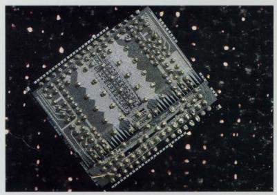
A combination of technology, innovation in hardware, microcode, and software delivers a balanced system to meet your requirements for capacity, function, and high performance in IBM large systems. The new double-density Read Only Storage (ROS) chip — which is 36% faster and 21% smaller than the previous chip — significantly increases the microcode capability of the enhanced 3090 models.
