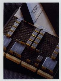
Two megabytes of memory are packaged on one card in the 3090 expanded storage. Each small module contains an IBM onemillion-bit memory chip.
