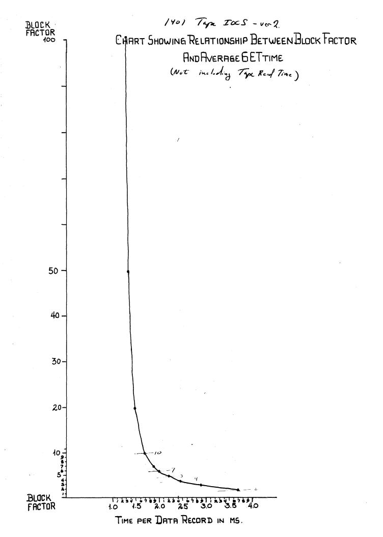
IBM 1401 TAPE IOCS TIMING CALCULATION FORMULAS
