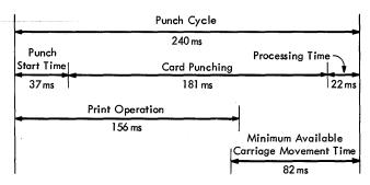
Figure 12. Write and Punch Operation—IBM 1403, Model 6, and IBM 1402, Models 4 and 5
