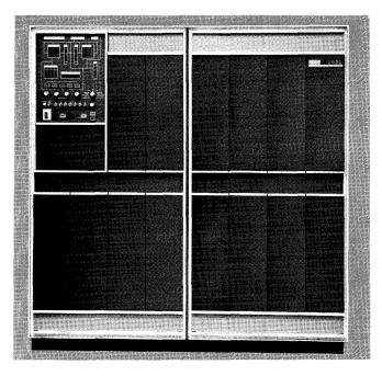
Figure 2. IBM 1401 Processing Unit, Model G
