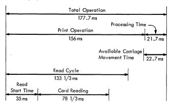
Figure 10. Write and Read Operation—IBM 1403 Printer, Model 6, and IBM 1402, Models 4 and 5
