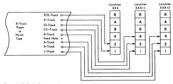
Figure 31. Eight-Track Tape Punching to Bit-Pattern Translation
