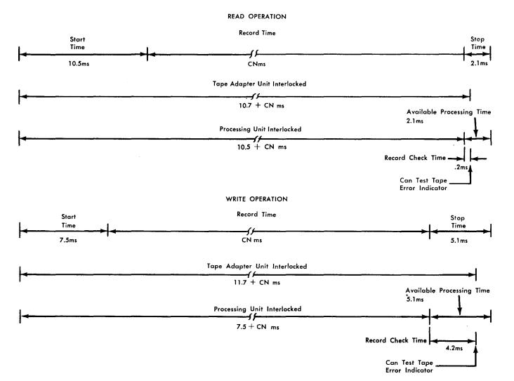
Figure 19. IBM 729, Model V, Read-Write Operation Timings
