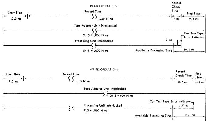
Figure 53. IBM 7335 Read-Write Operation Timing
