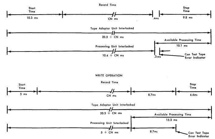
Figure 21. IBM 7330 Read-Write Operation Timings
