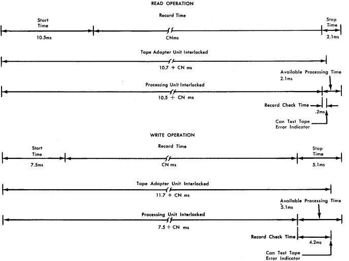
Figure 17. IBM 729, Model II, Read-Write Operation Timings
