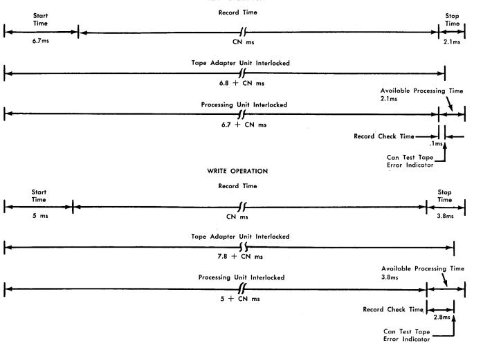
Figure 20. IBM 729, Model VI, Read-Write Operation Timings
