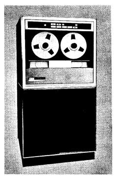
Figure 2. IBM 7330 Magnetic Tape Unit
