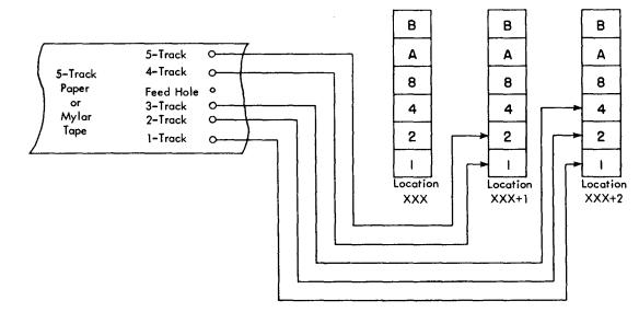
Figure 35. Five-Track Tape Punching to Bit-Pattern Translation
