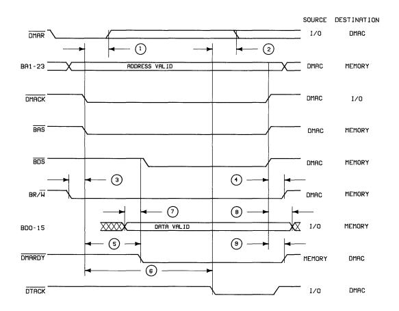
Figure 7. DMA Input Cycle Timing
