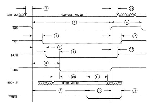
Figure 4. Write Cycle Timing
