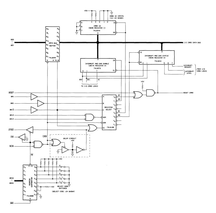
Figure 11. Example Data-Transfer Interface Design
