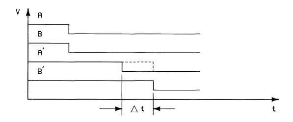
Figure 2. Origins of Signal Skew
