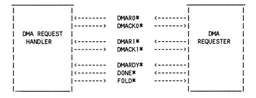
Figure 1c. Direct-Memory Access System Elements
