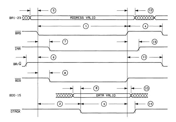
Figure 3. Read Cycle Timing
