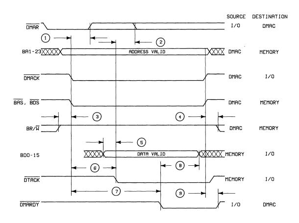
Figure 6. DMA Output Cycle Timing
