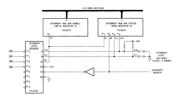
Figure 12. Example Interrupt Interface Design
