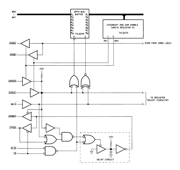
Figure 13. Example DMA Interface Design
