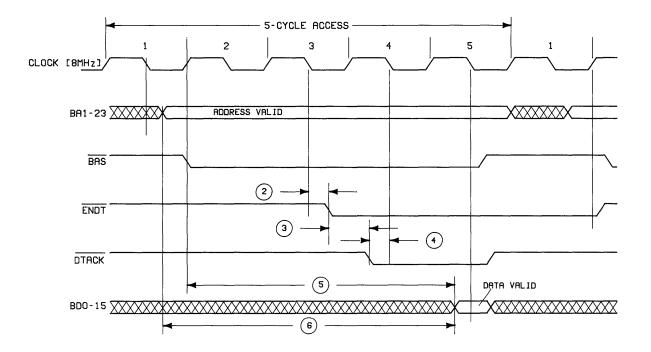
Figure 5. Enable DTACK Timing
