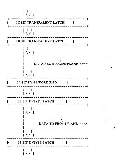
The input and output of the data path are the same, the 18 bit wide buffered version of the CIO backplane data lines, BD[15:0] and CDP[1:0] The output of the data path can not drive the BD[15:0]/CDP[1:0] lines at the same time as any other device on these lines.
