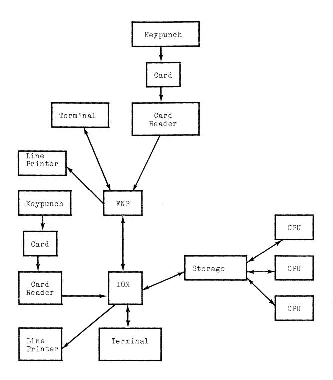
Figure 1-1. Components of Multics Hardware
