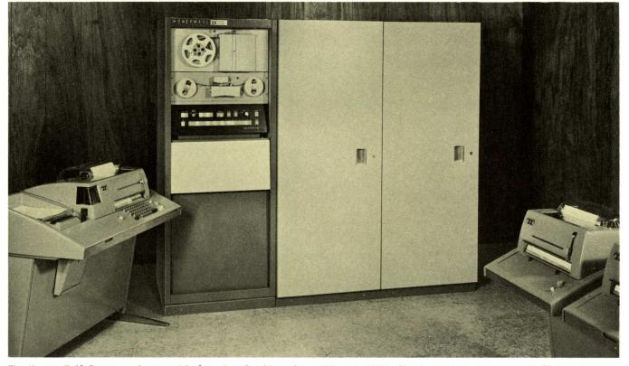
The Honeywell 20 System, rack-mounted in from 2 to 7 cabinets for industrial installations, is fully operational from 32 to  $120^{\circ}$ F. Cabinets are 70" high, 27" wide and 27" deep. Typical small system requires
