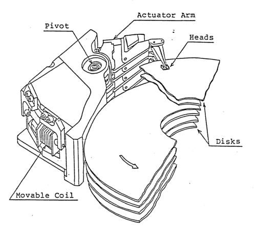
Figure 2-3 Actuator Arm Assembly
