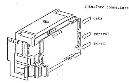
Figure 3-1 DK512 PC Boards and Interface Connectors
