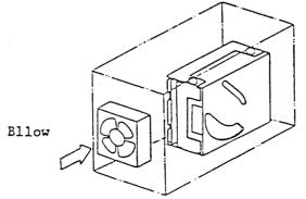
Figure 3-4 An Example of Forced Cooling
