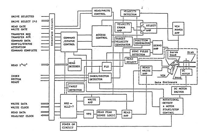
Figure 5-1 SERIAL Mode Block Diagram
