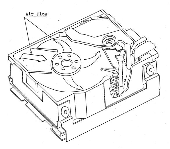
Figure 2-4 Air Circulation Inside Head and Disk Assembly
