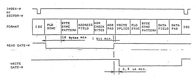
Figure 5-6 WRITE GATE Timing When Writing Data
