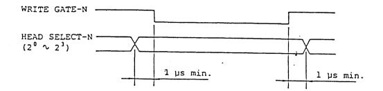
Figure 5-8 WRITE GATE Timing with HEAD SELECT
