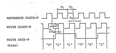
$T_{1} = 102.8 \text{ ns} + 8 \text{ ns}$   $T_{2} = T_{1}/2$   $T_{3} = T_{4}/2 + 20 \text{ ns}$   $T_{D} = 2T_{1}$  $T_{4} = 102.8 + 8 \text{ ns}$
