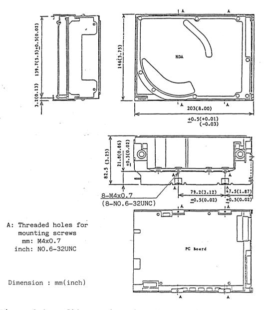
Figure 3-3 DK512 Mounting Dimensions: Side and Top Views
