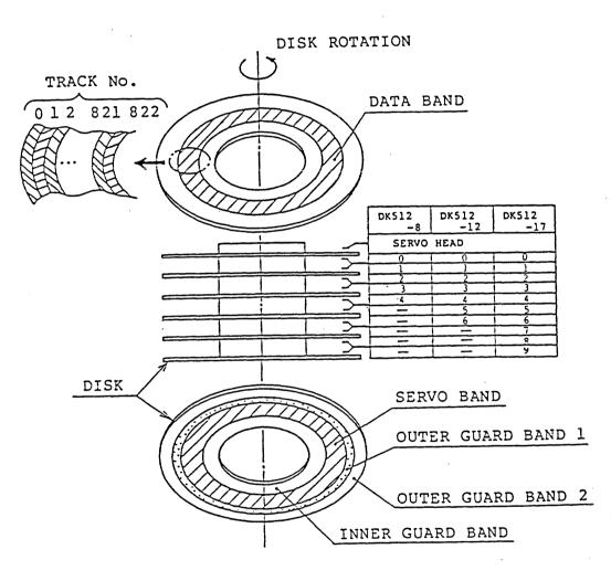
Figure 2-5 Head and Cylinder Address
