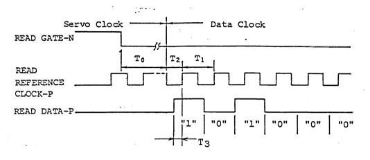
$T_0 = 4$  bytes  $T_1 = 102.8$  ns + 10 ns  $T_2 = T_{1/2} + 10$  ns  $T_3 = T_{1/2} + 15$  ns
