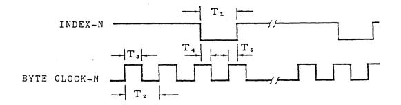
$T_1 = 0.8 \pm 0.2 \mu s$   $T_2 = T_1$   $T_3 = T_{1/2}$  $T_4 = T_5 = T_{3/2}$
