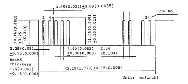
Figure 3-8 Control Cable B Connector J1
