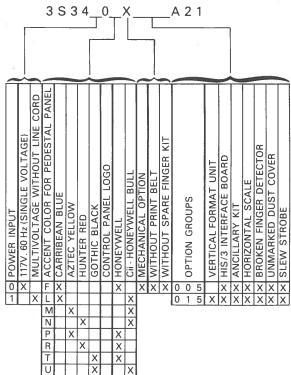
Figure 1-1 Honeywell Information System TermiNet 340 Printer Model Number Code Chart.
