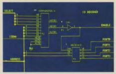
Designs created with the DASH Schematic Designer system are automatically converted to a CADAT<sup>™</sup> circuit description file using the pin list provided by DASH. This schematic depicts a simple Address Decoder of a peripheral device.
