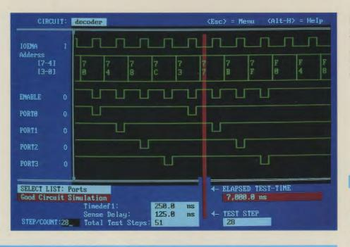
By looking at the address bus lines on the waveform display, you can easily see whether the circuit is enabling the correct ports given the inputs. Select the sequence of the displayed signals and how you want them grouped.
