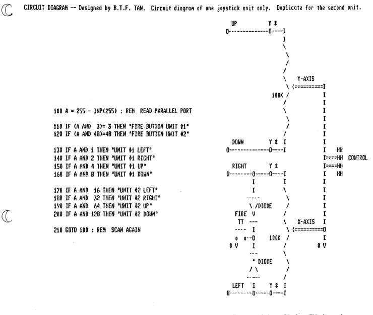
\$ note : tied to +5V via a 50K ohm resistor \$ note : tied to GROUND
