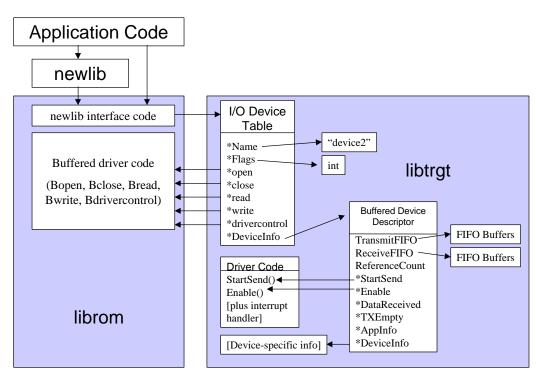
Figure 4.2: Buffered I/O device implementation
