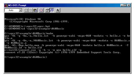
Figure 2.1: compiling 'Hello world' for the MDP860Basic board
