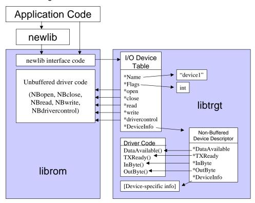
Figure 4.1: Non-buffered I/O device implementation
