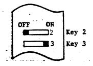
The figure at left shows the configuration for sending the Sector Signal.
