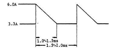
Note) The peak current (6A) in the A section flows only 3 or 4 times during one seek.
