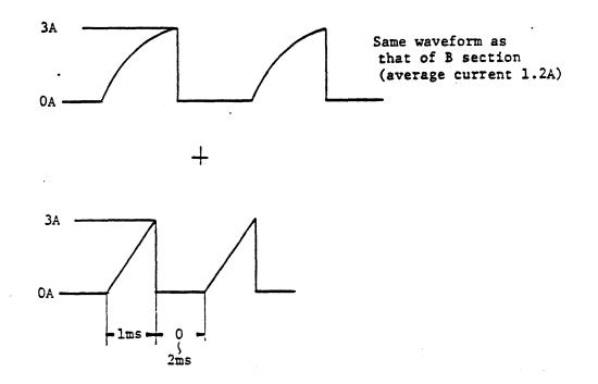
The waveform of the C section is obtained by superimposing the above two waveforms asynchronously.
