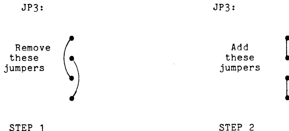
Figure 7. Reversing the order of the EVEN and ODD bytes.
