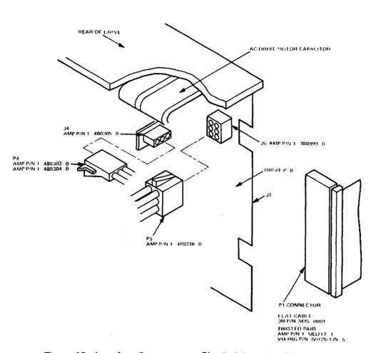
Figure 16. Interface Connectors – Physical Location Diagram
