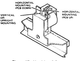
Figure 17. Head Load Actuator Mounting Prerequisites
