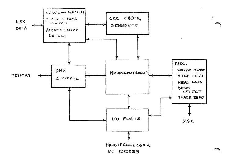
Figure I. FDC-I Block Diagram.
