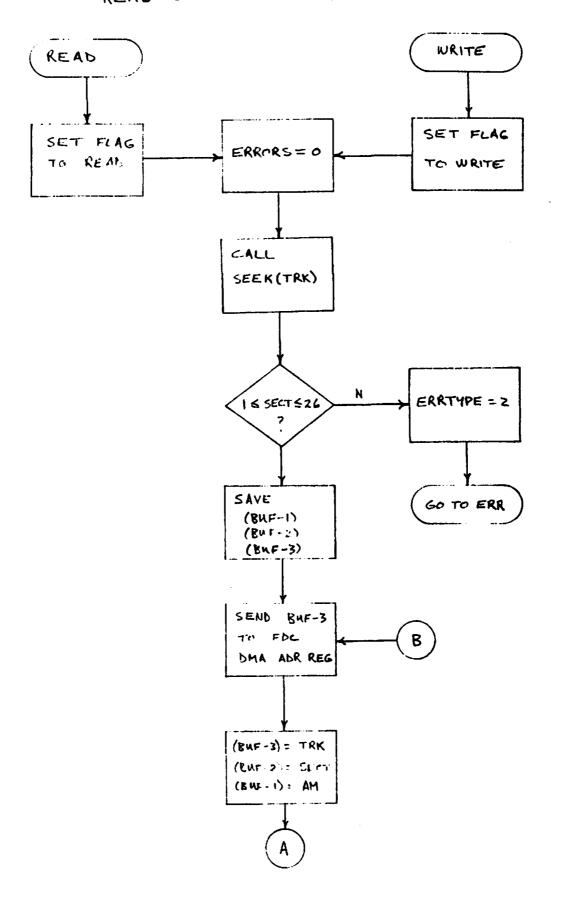
Figure 7. Subroutines READ and WRITE.
