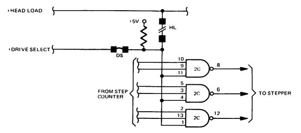
Figure 23. Stepper Motor Enable Circuit
