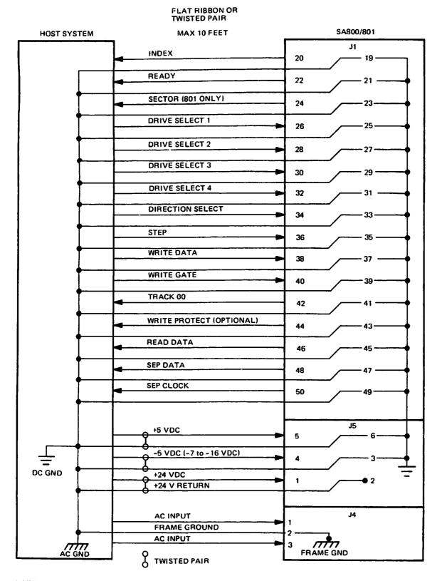
NOTE: Not shown are the nine Alternate I/O connections. The connections for these lines are on pins 2, 4, 6, 8, 10, 12, 14, 16, and 18. Signal return for these lines are on pins 1, 3, 5, 7, 9, 11, 13, 15, 17, and 19 respectively. Reference section 7 for uses of these lines.
