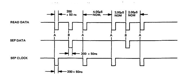
A = LEADING EDGE OF BIT MAYBE ± 400 ns FROM ITS NOMINAL POSITION. B = LEADING EDGE OF BIT MAYBE ± 200 ns FROM ITS NOMINAL POSITION.
