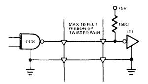
Figure 10. Interface Signal Driver/Receiver
