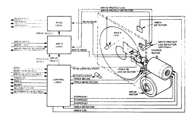
Figure 2. SA800/801 Functional Diagram
