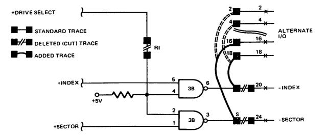
Figure 26. Radial Index/Sector Circuit
