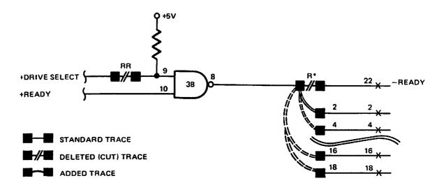
Figure 25. Radial Ready Circuit
