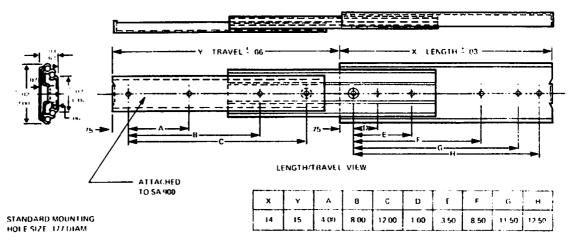
Figure 19. Slide Mounting Dimensions
