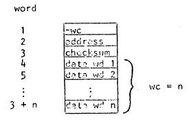
The two's complement of the number of data words in the block is given in the first word (therefore bit 0 is a 1). Mormally 16 data words will be punched per data block. However, the .END and .LOC pseudo-ops may cause
