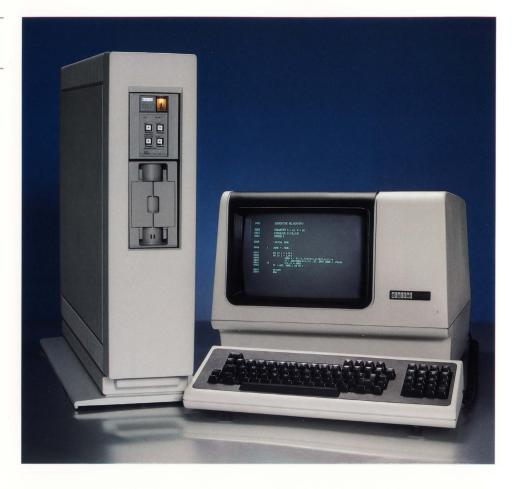
ance. Part of the solution was to emulate some little-used instructions and data types using microcode-assisted software. The CPU hardware is especially designed to make this emulation most efficient, so that MicroVAX I can give you VAX performance at a size and price never before seen in a VAX system.
