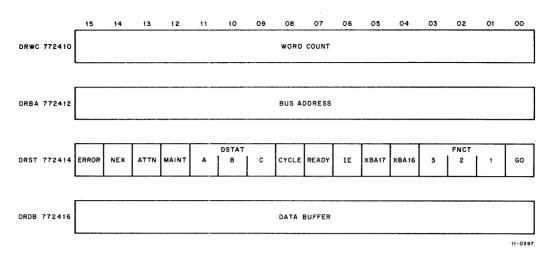
Figure 2-1 Register Assignments
