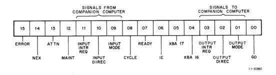
Figure C-5 DRST Register Assignments
