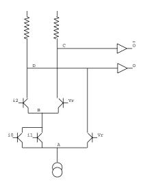
Figure 2: gate for  $F = (i_0 + i_1)\overline{i_2}$
