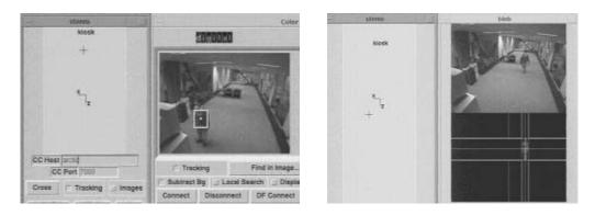
Figure 2: Sample output from the color tracking (left) and motion blob tracking (right) modules. Images were obtained from the right camera of the stereo pair. The left hand portion of each display shows a plan view of the scene with a cross marking the 3D location of the individual projected onto the ground plane.
