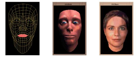
Figure 3: DECface rendered in wireframe (left), as a texture mapped anonymous face (middle) and a female face (right).
