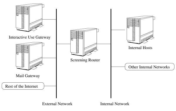
Figure 1: Typical Firewall Configuration
