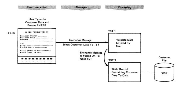
Figure 3-6 Transfer of the Exchange Message
