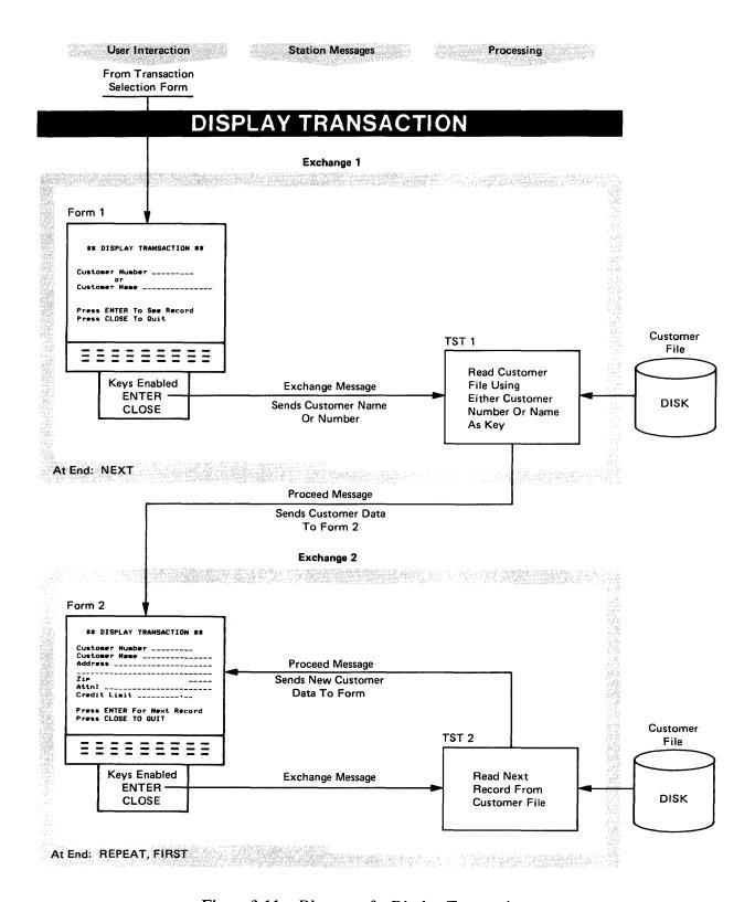
Figure 3-11 Diagram of a Display Transaction
