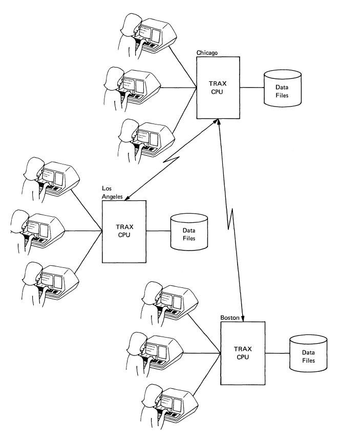
Figure 1-11 TRAX to TRAX Data Communication
