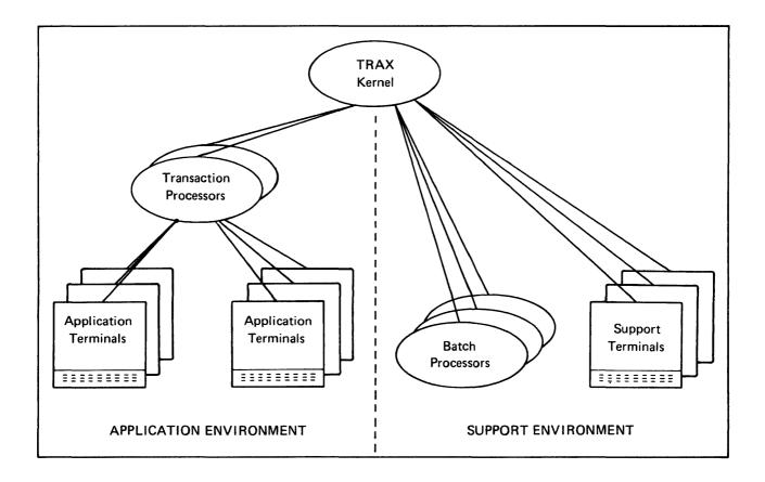
Figure 1-4 TRAX System Structure
