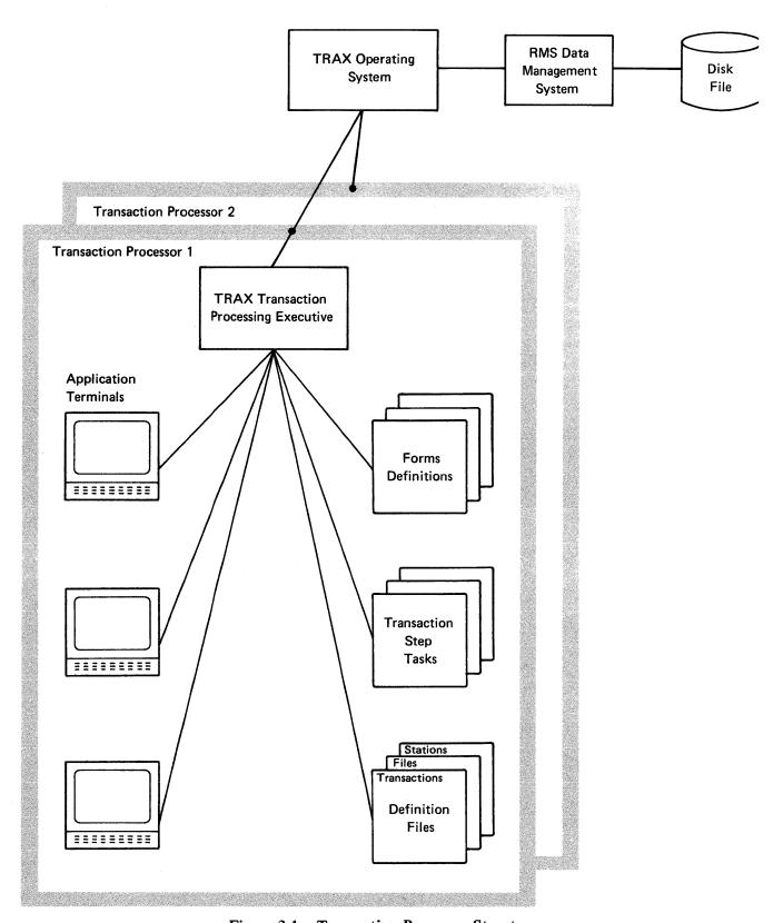
Figure 3-1 Transaction Processor Structure
