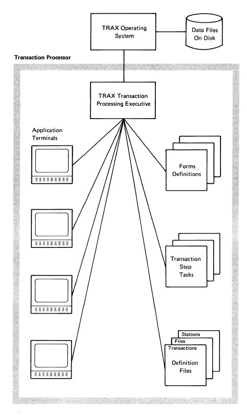
Figure 1-9 Transaction Processor Structure
