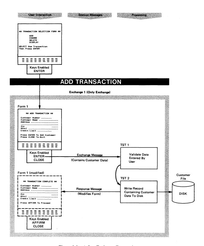
Figure 3-8 A One Exchange Transaction
