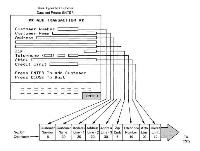
Figure 3-5 Creation of a Typical Exchange Message
