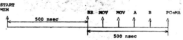
For this subroutine it took four Source-Destination instructions and required approximately 1.0 used to perform the A+B-B transfer. A more time-consuming computation would be a Memory Register to Destination Register transfer. The subroutine computation to accomplish this is as follows:
